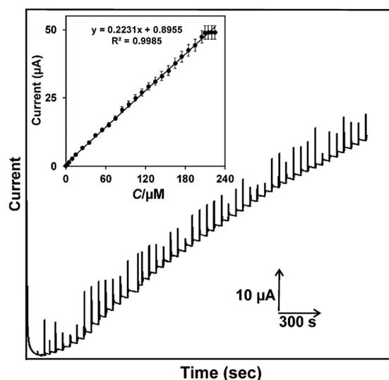
**Figure 9.** Amperometric  $i-t$  response of the GR-CMF/laccase modified SPCE for different concentration additions (0.2 to 224.7  $\mu\text{M}$ ) of CC into the constantly stirred 0.1 M sodium phosphate buffer pH 5.0; Working potential = +0.4 V. Inset is the linear plot for the amperometric current response vs. [CC].
