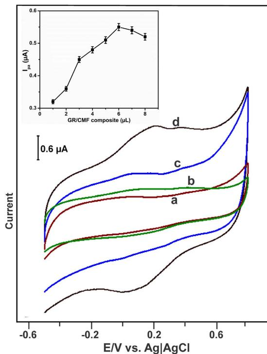
**Figure 4.** Cyclic voltammetry response of laccase immobilized on bare SPCE (a), CMF/SPCE (b), GR/SPCE (c) and GR-CMF/SPCE (d) in pH 5.0 at a scan rate of 100 mV/s. Inset shows the effect of different drop coated amount of GR/CMF composite vs. anodic redox peak current response of immobilized laccase on GR/CMF composite.
