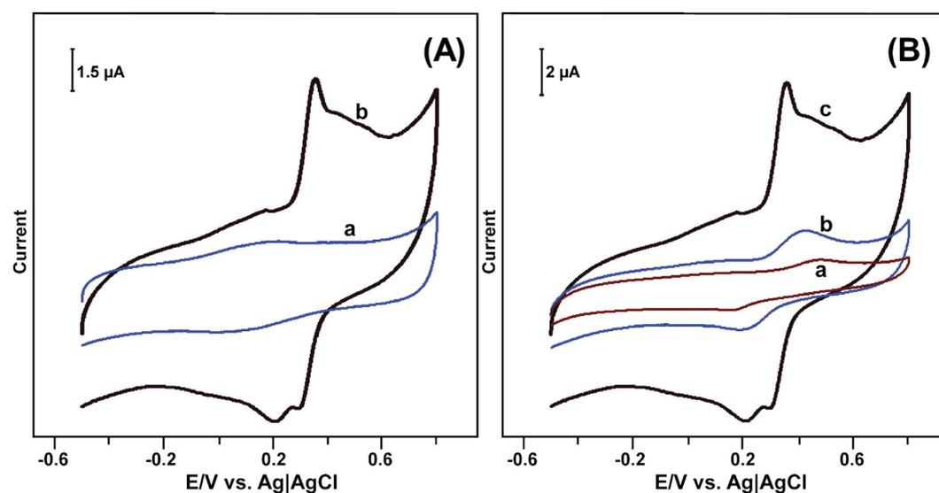
**Figure 7.** (A) Cyclic voltammetric response obtained for GR-CMF/laccase modified SPCE in the absence (a) and presence (b) of 50  $\mu\text{M}$  CC in pH 5 at a scan rate of 100 mV/s. (B) At similar conditions, the cyclic voltammetry response of CMF (a), GR-CMF (b) and GR-CMF/laccase (c) modified SPCEs towards 50  $\mu\text{M}$  CC.
