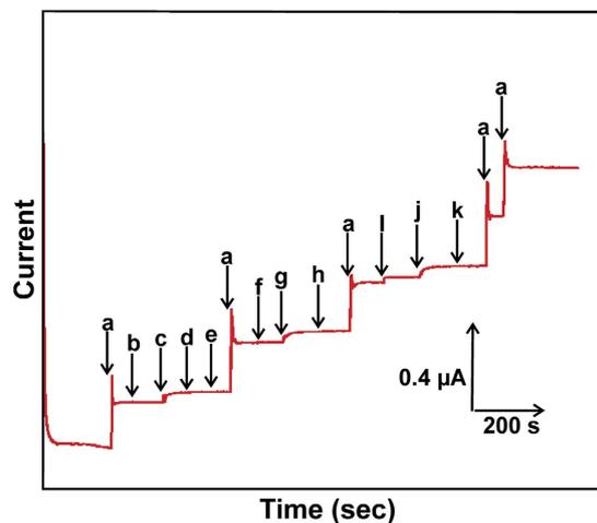
**Figure 10.** Amperometric *i-t* response of the biosensor for the addition of 1  $\mu\text{M}$  CC (a) and 50  $\mu\text{M}$  additions of hydroquinone (b), dopamine (c), resorcinol (d), phenol (e), 2-amino phenol (f), pyrogallol (g), caffeic acid (h), gallic acid (i), catechin (j) and phloroglucinol (k) into the constantly stirred 0.1 M sodium phosphate buffer pH 5.0.
