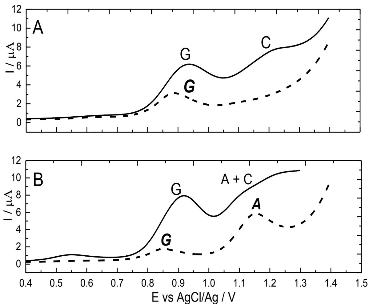
Fig. ESI-3. SWV responses of 300  $\mu\text{M}$  5'-CGCGCG-3' (plot A solid line); 300  $\mu\text{M}$  5'-AAACGC-3' (plot B, solid line); 18  $\mu\text{M}$  of dGMP from the enzymatically treated 5'-CGCGCG-3' (plot A, dashed line) and 18  $\mu\text{M}$  of dAMP from the enzymatically treated 5'-AAACGC-3' (plot B, dashed line). 0.1 M acetate buffer solution pH 5.0.
