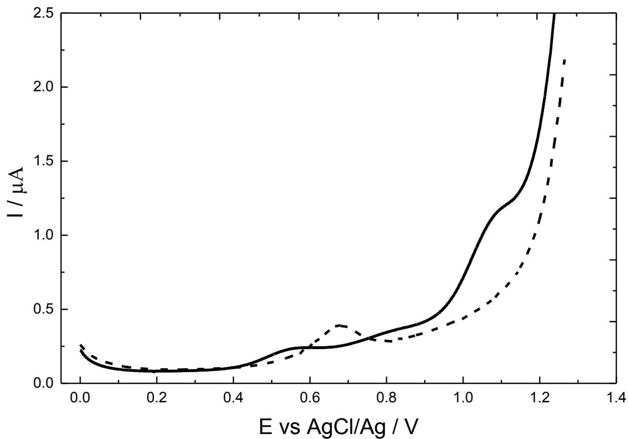
Fig. ESI-2. SWV response of 300  $\mu\text{M}$  polyC (solid line) and 18  $\mu\text{M}$  dCMP from the enzymatically treated polyC (dashed line) in 0.1 M acetate buffer solution pH 5.0.
