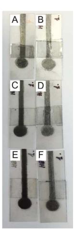
**Figure S4.** Optical images of PDEs fabricated using different batches of HB pencils, designated as PDE1 (**A**); PDE2 (**B**); PDE3 (**C**); PDE4 (**D**); PDE5 (**E**) and PDE6 (**F**), respectively.
