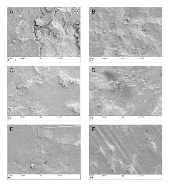
**Figure S6.** SEM images of different PDEs fabricated using different batches of HB pencils (boxes 1 to 6) on plastic substrates: PDE1 (**A**); PDE2 (**B**); PDE3 (**C**); PDE4 (**D**); PDE5 (**E**) and PDE6 (**F**), respectively.
