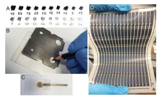
**Figure 1.** Different pencil grades and their graphite deposition (**A**); fabrication of Pencil-drawn Electrodes (**B**); a typical final Pencil-drawn Electrode (**C**) and an image of a sheet of screen-printed electrodes fabricated via the screen-printing process (**D**).
