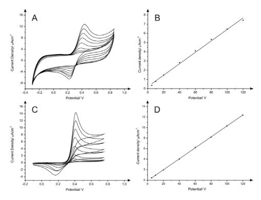
**Figure 4.** Cyclic voltammograms and calibration curves of acetaminophen using PDE1 drawn 60 times with HB pencil from Box 1 (**A**) and (**B**) and screen-printed electrodes (**C**) and (**D**) in 0.1 M pH 7.4 PBS/0.1 M KCl Each data point shown in (**B**) and (**D**) is the average and standard deviation of the replicates (N = 3). Scan rate: 5 mV·s<sup>-1</sup>.
