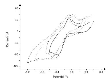
**Figure 2.** Typical cyclic voltammograms recorded with 1 mM hexaammineruthenium(III) chloride/0.1 M KCl using PDE1 (HB pencil, Box 1) drawn 15 (dotted line), 30 (dashed line), 60 (solid line) and 100 (dashed dotted line) times. Scan rate:  $50 \text{ mV} \cdot \text{s}^{-1}$ .
