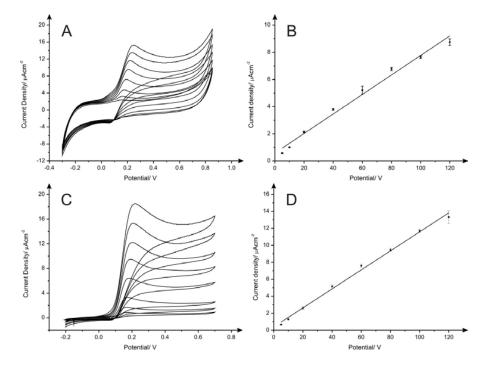
**Figure 3.** Cyclic voltammograms and calibration curves of dopamine using PDE1 drawn 60 times with HB pencil from Box 1 (**A**) and (**B**) and screen-printed electrodes (**C**) and (**D**) in 0.1 M pH 7.4 PBS/0.1 M KCl. Each data point shown in (**B**) and (**D**) is the average and standard deviation of the replicates (N = 3). Scan rate: 5 mV·s<sup>-1</sup>.
