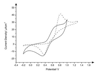
**Figure S5.** Comparison of cyclic voltammograms using PDE1 (solid line) and SPE (dotted line) recorded in 1 mM ammonium iron(II) sulphate/0.2 M HClO<sub>4</sub>. Scan rate:  $5 \text{ mV} \cdot \text{s}^{-1}$ .
