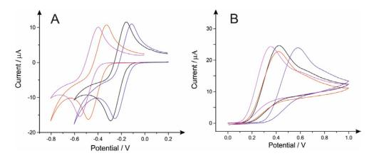
**Figure S8.** Typical cyclic voltammograms recorded using PDE1 (drawn 60 times) towards 1 mM hexaammineruthenium(III) chloride/0.1 M KCl (**A**) and 1 mM uric acid/0.1 M PBS (**B**), utilising screen-printed Ag/AgCl (black line), screen-printed carbon (red line), saturated calomel electrode (purple line) and pencil-drawn graphite references (pink line). Scan rate: 50 mV·s<sup>-1</sup>.
