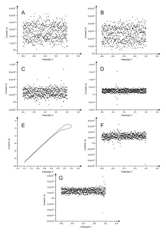
**Figure S1.** Cyclic voltammograms of 60 times drawn PDEs fabricated applying different pencil grades B (**A**); 2B (**B**); 3B (**C**); 4B (**D**); 7B (**E**); 8B (**F**) and 9B (**G**) from Box 1. Redox probe: hexaammineruthenium(III) chloride/0.1 M KCl. Scan rate:  $5 \text{ mV} \cdot \text{s}^{-1}$ .
