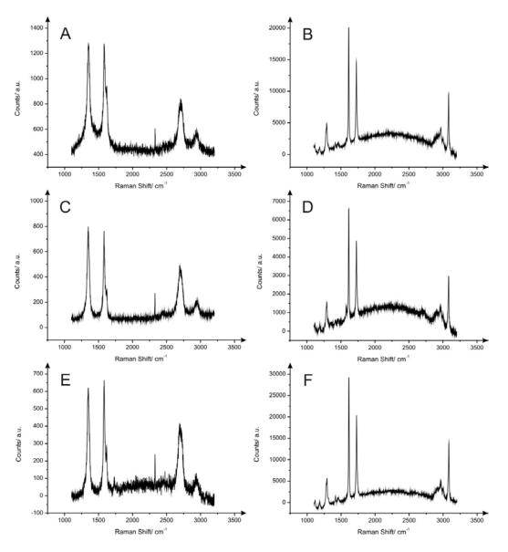
**Figure S7.** Raman results for PDEs (boxes 1–6) fabricated using different batches of HB pencils, designated as PDE1 (**A**); PDE2 (**B**); PDE3 (**C**); PDE4 (**D**); PDE5 (**E**) and PDE6 (**F**), respectively.
