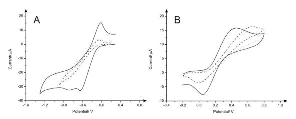
**Figure S3.** Comparison of cyclic voltammograms recorded for PDEs fabricated using HB pencils from boxes 1, 3 and 5, respectively, in 1 mM hexaammineruthenium(III) chloride (**A**) and 1 mM potassium ferrocyanide(II) (**B**) redox probes/0.1 M KCl. Scan rate:  $5 \text{ mV} \cdot \text{s}^{-1}$ . PDE1 (solid line), PDE3 (dashed line) and PDE5 (dotted line).
