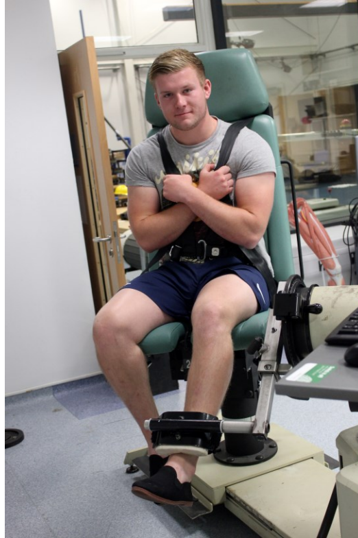
Figure 4. 2 The Cybex dynamometer and participant position.
