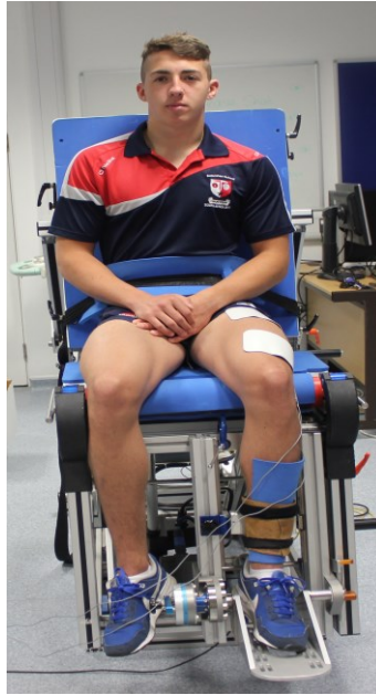
Figure 4. 3 Position of participant and placement of electrodes
