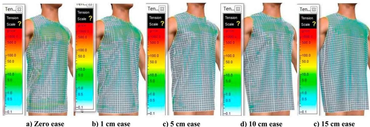
**Figure 7.** Tension maps on longer shirt from CAD system 2.
