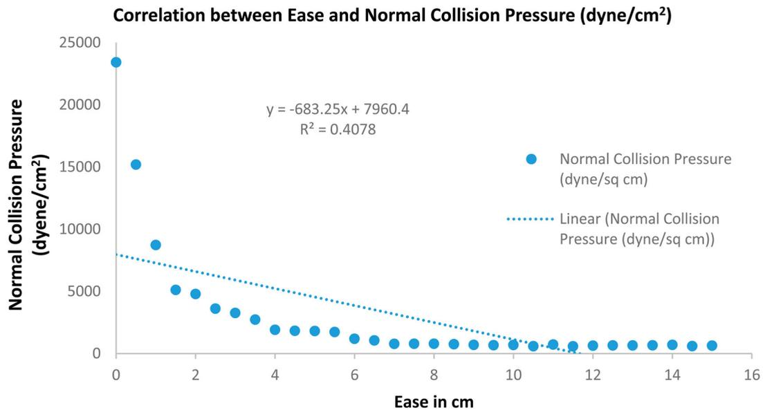
**Figure 6.** Correlation between ease and normal collision pressure in longer shirts.
