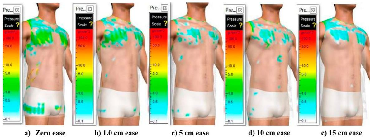
**Figure 8.** Pressure maps on longer shirt from CAD system 2.
