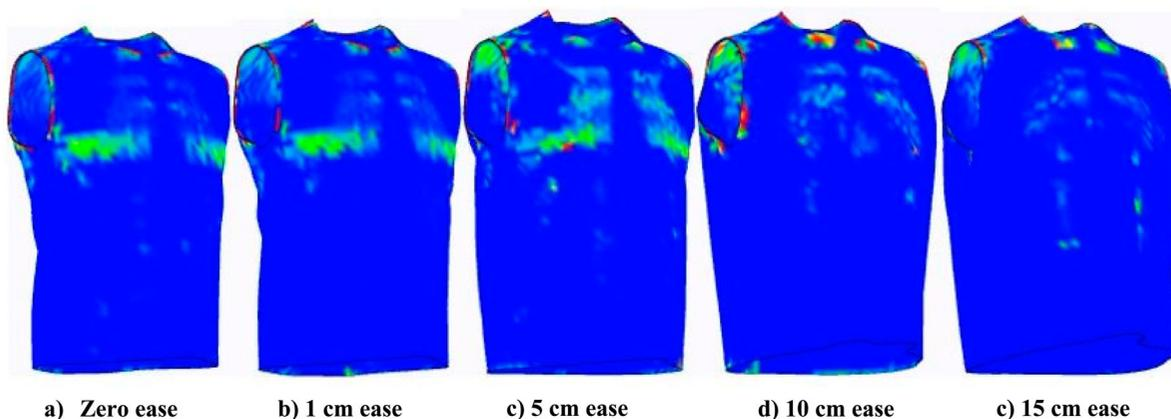
**Figure 13.** Collision pressure maps on the virtual shirt from shorter patterns.
