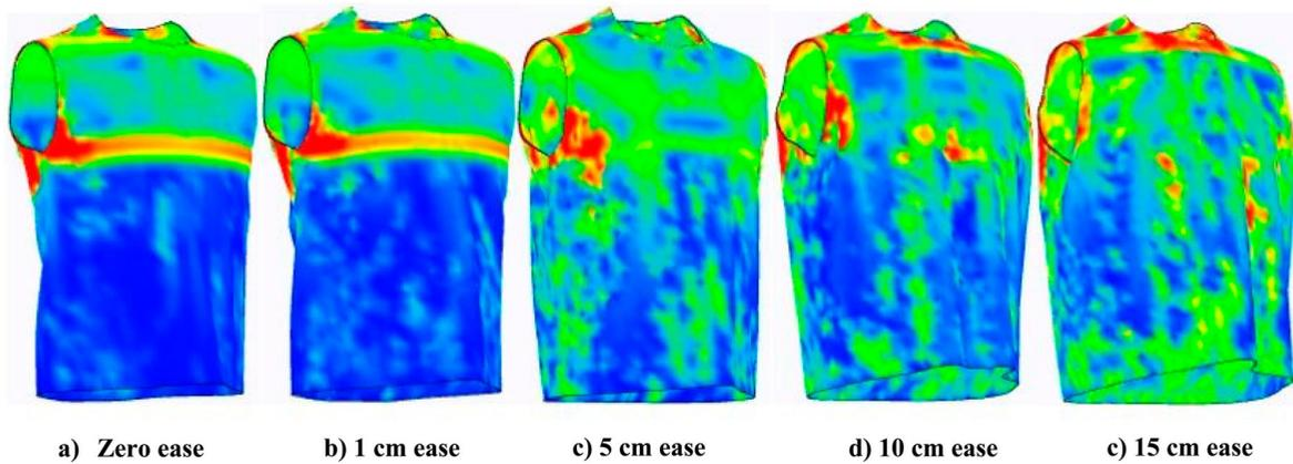
**Figure 9.** Tension maps on the virtual shirts from shorter pattern pieces with varying eases.
