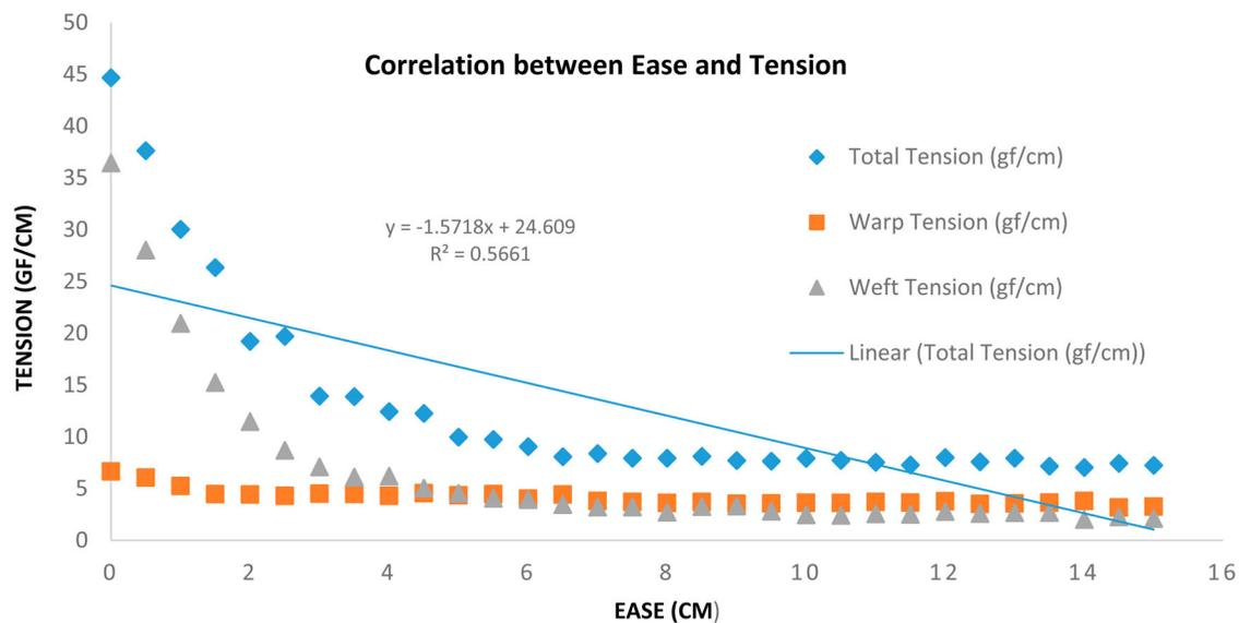
**Figure 2.** Correlation between ease in pattern and tension in virtual fabric in the longer shirts.
