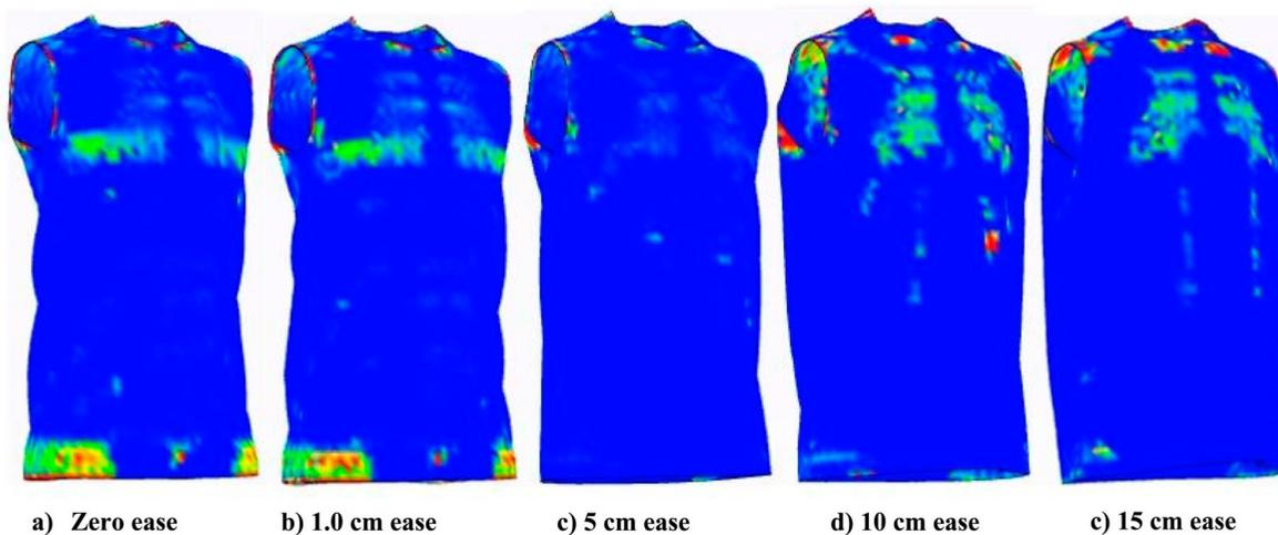
Figure 5. Collision pressure maps on the virtual shirt from longer patterns.
