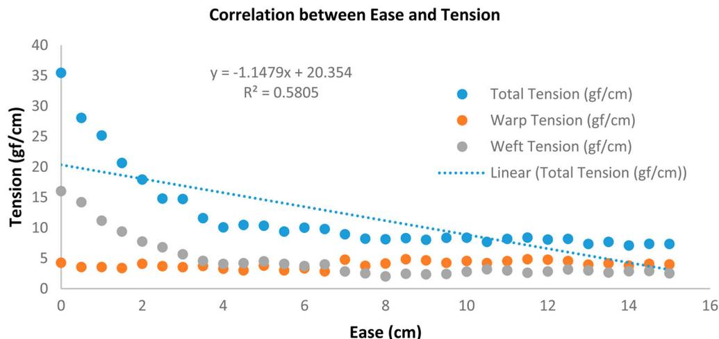
**Figure 10.** Correlation between ease in pattern and tension in virtual fabric of the shorter shirts.
