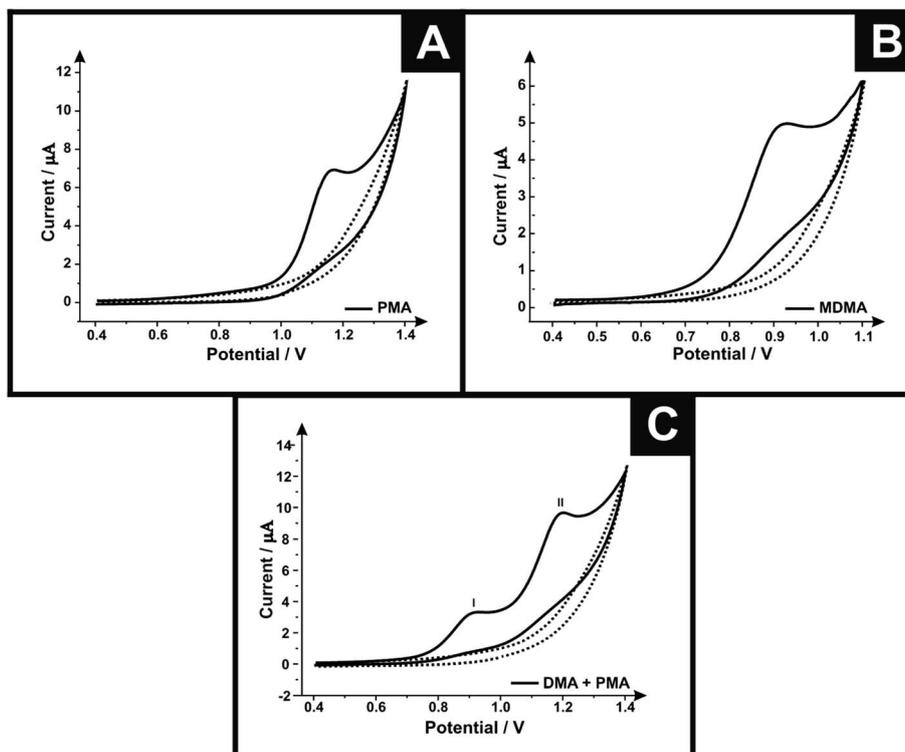
Fig. 1 Cyclic voltammograms of SPE (A) in presence ( $500 \mu\text{g mL}^{-1}$ ) and absence of PMA, (B) in presence ( $250 \mu\text{g mL}^{-1}$ ) and absence of MDMA and (C) in presence ( $250 \mu\text{g mL}^{-1}$ )/( $500 \mu\text{g mL}^{-1}$ ) and absence of MDMA/PMA in PBS (pH 7) (scan rate:  $100 \text{ mV s}^{-1}$ ).
