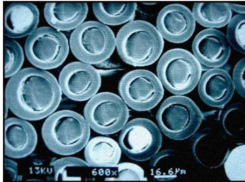
Figure 8 Outlast® technology polyester fibre cross section with thermocules
