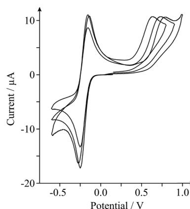
Fig. 3 Cyclic voltammograms obtained in pH 7 PBS (with 0.1 M KCl) containing 0.5 mM NADH and 0.5 mM  $\text{Ru}(\text{NH}_3)_6^{2+/3+}$  (internal standard) at three different double-layered defect-abundant graphene electrodes to investigate the inter-repeatability. Scan rate shown:  $100 \text{ mV s}^{-1}$  (vs. SCE).
