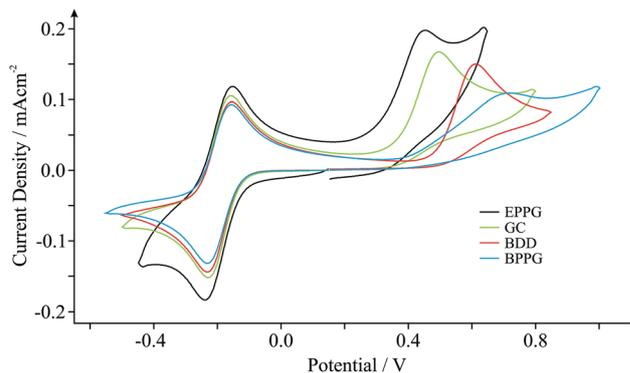
Fig. 1 Cyclic voltammograms obtained in pH 7 PBS (with 0.1 M KCl) containing 0.5 mM NADH and 0.5 mM  $\text{Ru}(\text{NH}_3)_6^{2+/3+}$  (internal standard) at EPPG (black), GC (green), BDD (red) and BPPG (blue) electrodes. Scan rate shown: 100  $\text{mV s}^{-1}$  (vs. SCE).
