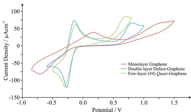
Fig. 2 Cyclic voltammograms obtained in pH 7 PBS (with 0.1 M KCl) containing 0.5 mM NADH and 0.5 mM  $\text{Ru}(\text{NH}_3)_6^{2+/3+}$  (internal standard) at monolayer graphene (red), double-layer defect-graphene (blue) and quasi-graphene (green) electrodes. Scan rate shown:  $100 \text{ mV s}^{-1}$  (vs. SCE).
