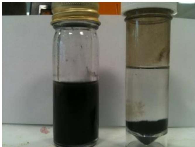
Figure 3.9b: On the left is the solution containing pH=4 HgS with the addition of Nafion while the right contains HgS nanoparticles at pH=2 left for 24 hours
