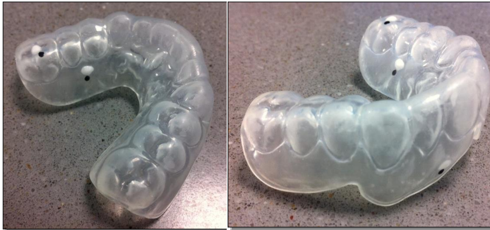
Figure 3-3 Markers placed onto the mouthguards (black points: original permanent marker anatomical measurement points, white points: barium markers).
