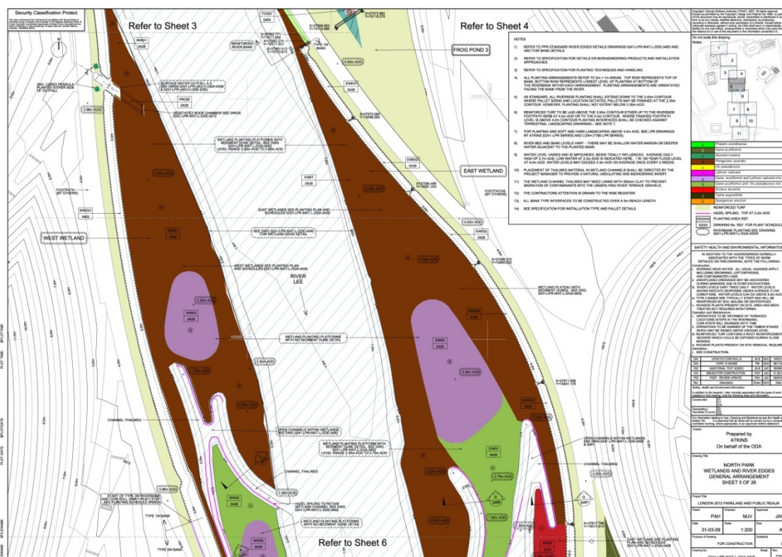
Figure 13: Atkins, Wet Woodland south outlet structure (sheet 2 of 3) sections London 2012 Olympic park infrastructure 29/7/09 Mike Vaughan. This drawing for contractors shows the locations were to plant along a river's edge, and contains information to create and maintain the surrounding wetlands, which has ability to maintain its form over time. Contractor WS Atkins conducted engineering for the Olympic Park for the London 2012 Olympic and Paralympic Games, in a large scale greening project for the Lower Lee Valley. Site analysis showed half a century of mixed industrial land use and contamination. Imported fill was also used to reclaim marsh land during the industrial revolution. Building waste from WW2 and rubbish tips also contributed towards the difficult site conditions. Around 2 million m 3 of cut and 2 million m 3 of fill were undertaken in the bulk earthworks operations, which predominantly retained on site. Two Soil hospitals were used to treat soil through physicochemical technology (Ian Mead et al. 2011, p.5).
