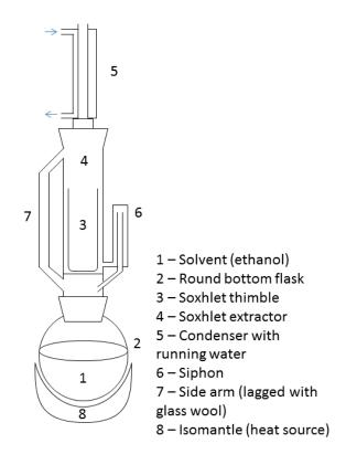
Figure 65. - Diagram of Soxhlet extraction equipment.
