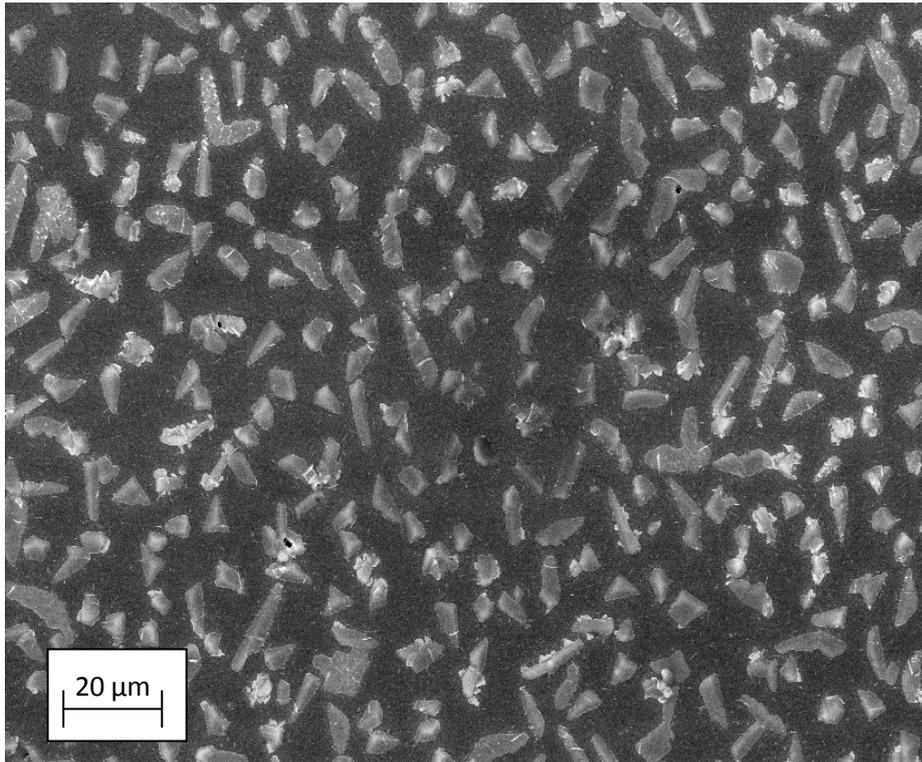
Figure 10.13: SEM top image of TiO<sub>2</sub> sample 5, deposited onto float glass, post-deposition annealed at 800°C.
