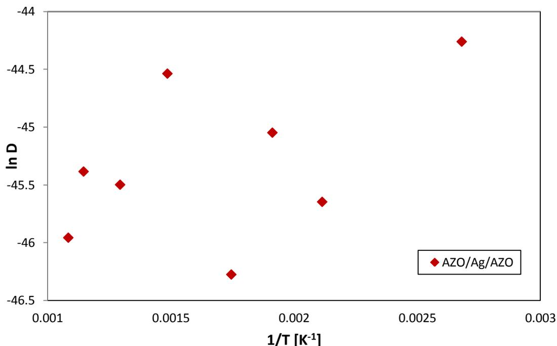
Figure 14.12: Arrhenius plot of Al-doped ZnO/Ag/Al-doped ZnO coating stack annealed at different temperatures.
