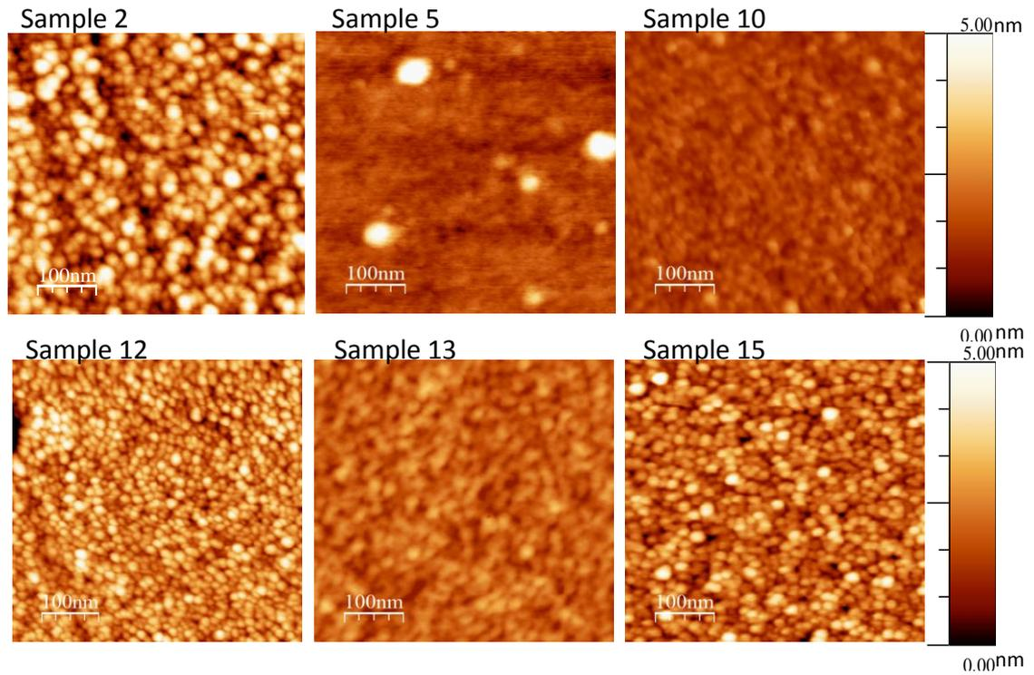
Figure 12.4: AFM images of six selected zinc stannate samples deposited onto float glass substrate.
