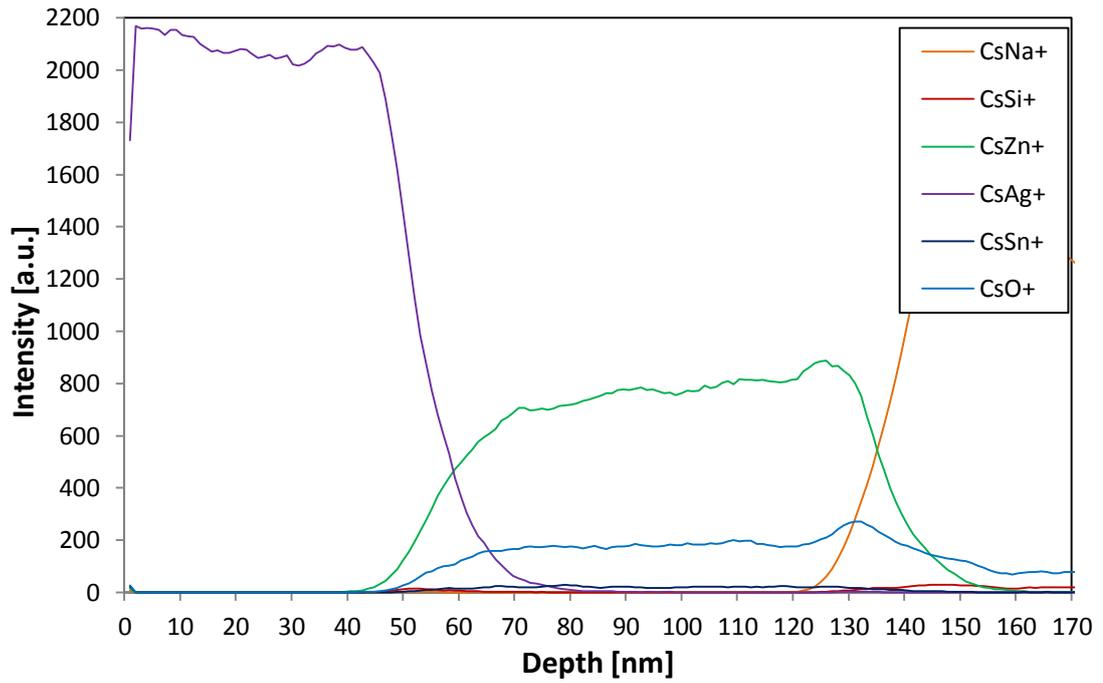
Figure 12.6: An example of TOF-SIMS depth profiling in as-deposited zinc stannate sample 17.
