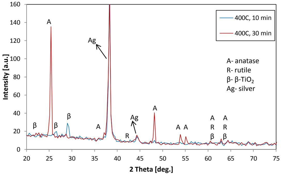
Figure 10.21: XRD diffractograms collected from TiO<sub>2</sub> annealed at 400°C for 10 minutes and 30 minutes respectively.
