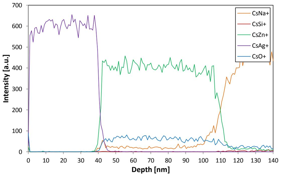
Figure 11.10: Example of TOF-SIMS profile collected from annealed Al-doped ZnO sample 3.1.
