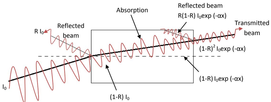
Figure 8.5: The beam fractions which are reflected, absorbed and transmitted through the material.
