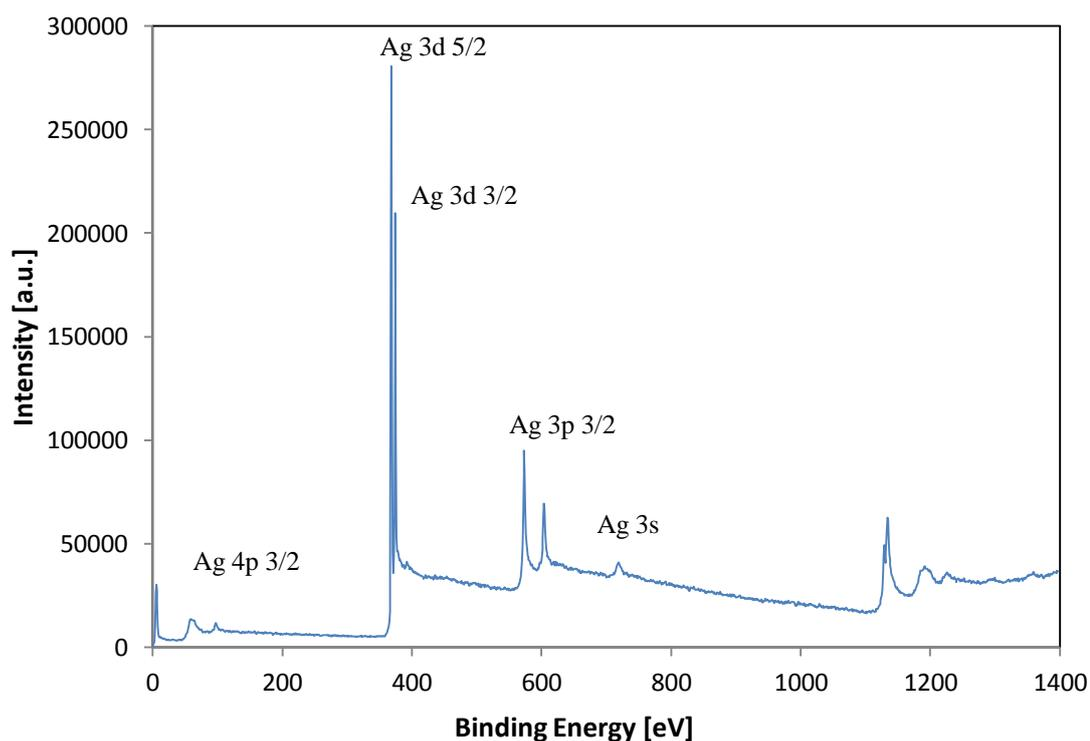
Figure 10.31: XPS spectrum collected for sample 6.1 after first sputter sequence (i.e. after first bombardment of the sample surface with Ar<sup>+</sup> gun to remove the material subjected to XPS depth profiling analysis).
