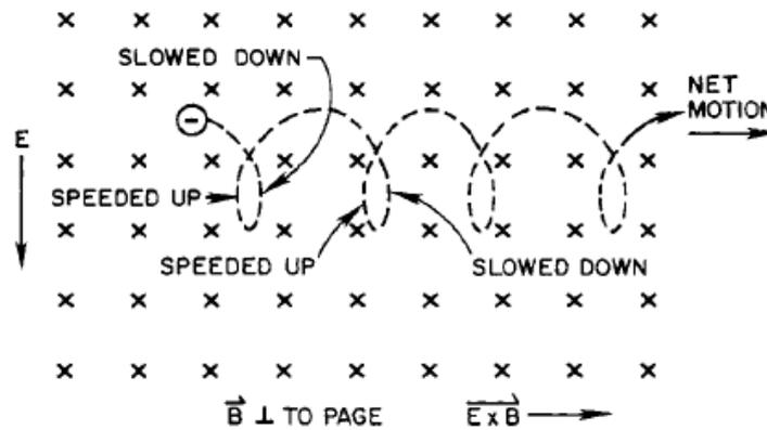
Figure 4.6: The motion of an electron in an electric and a magnetic field. The electric field is vertical, and the magnetic field is perpendicular to the plane of the page. [65]
