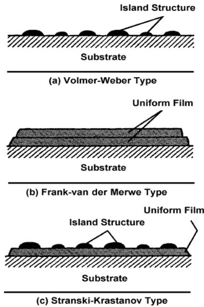
Figure 5.1: Schematic representation of different film growing techniques. [67]
