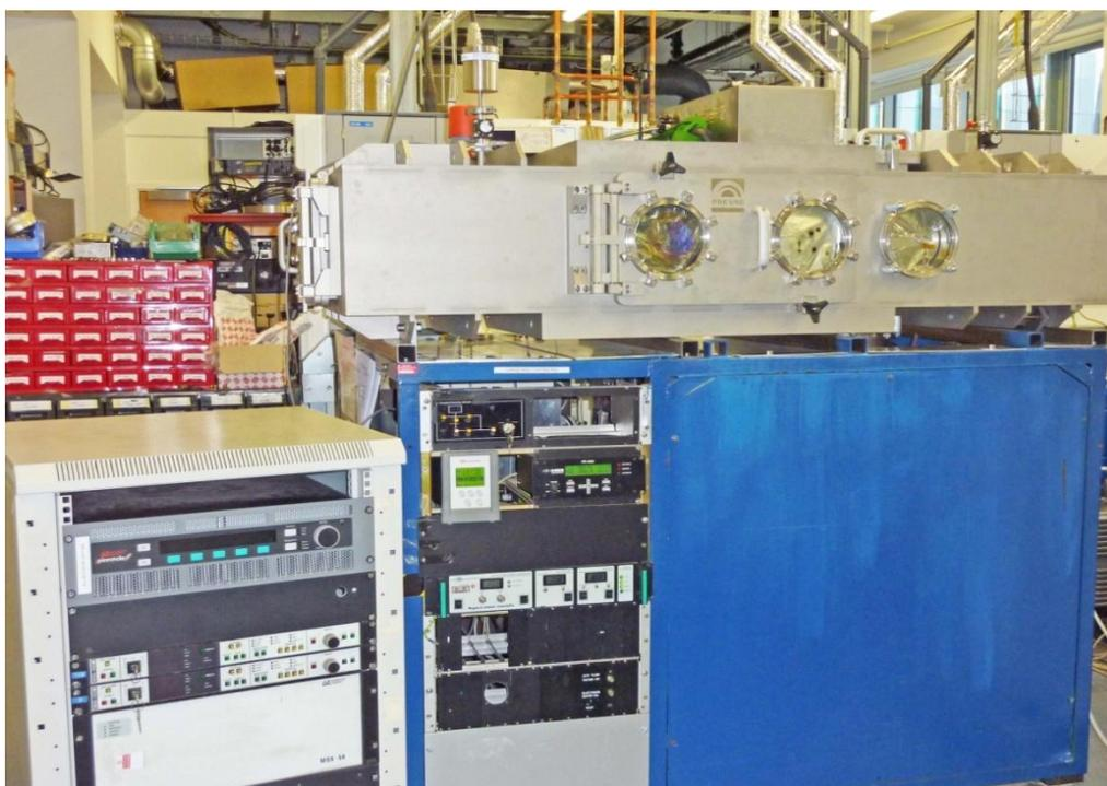
Figure 7.1: Large Area coating chamber (Prevac Sp. z.o.o.)
