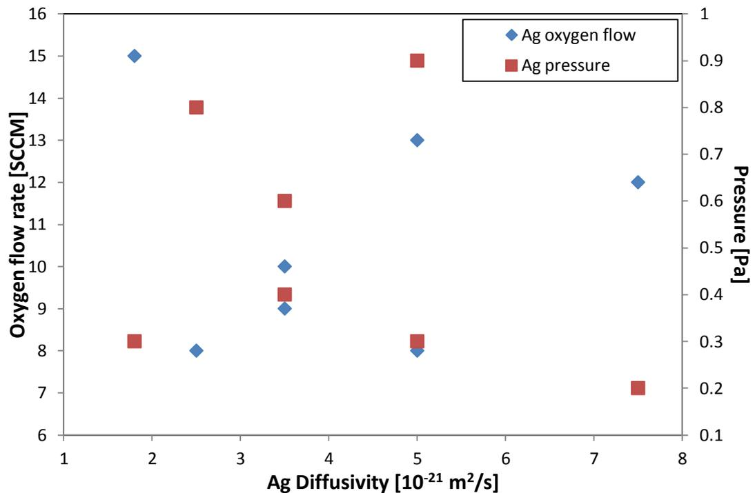
Figure 11.11: The dependency of silver diffusion values on operating pressure and oxygen flow during AZO samples deposition. Samples were post-deposition annealed at  $650^\circ\text{C}$ .
