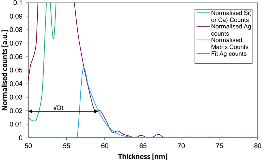
Figure 9.3: Ag counts fitted into Fick's second law analytical solution.
