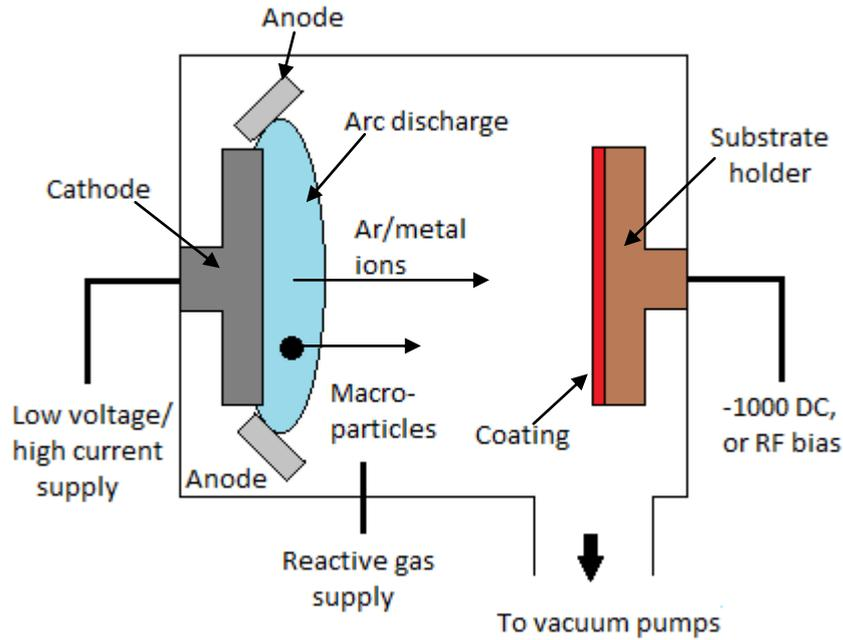
Figure 4.3: Schematic representation of cathodic arc evaporation system.
