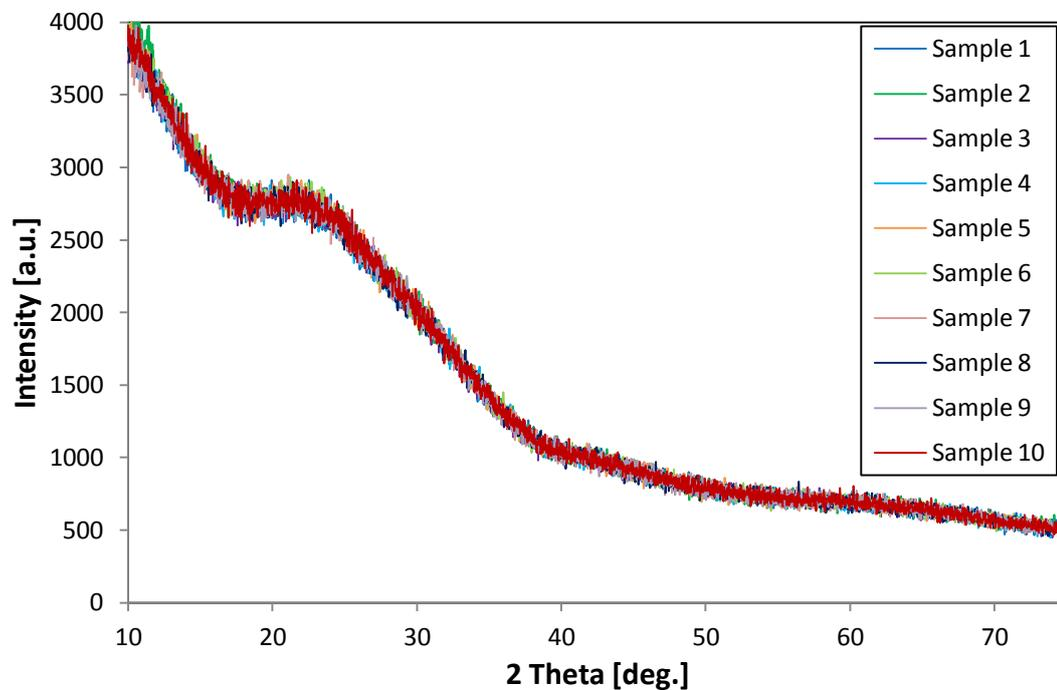
Figure 13.1: XRD spectra collected from ten  $\text{Si}_3\text{N}_4$  samples investigated in this work.
