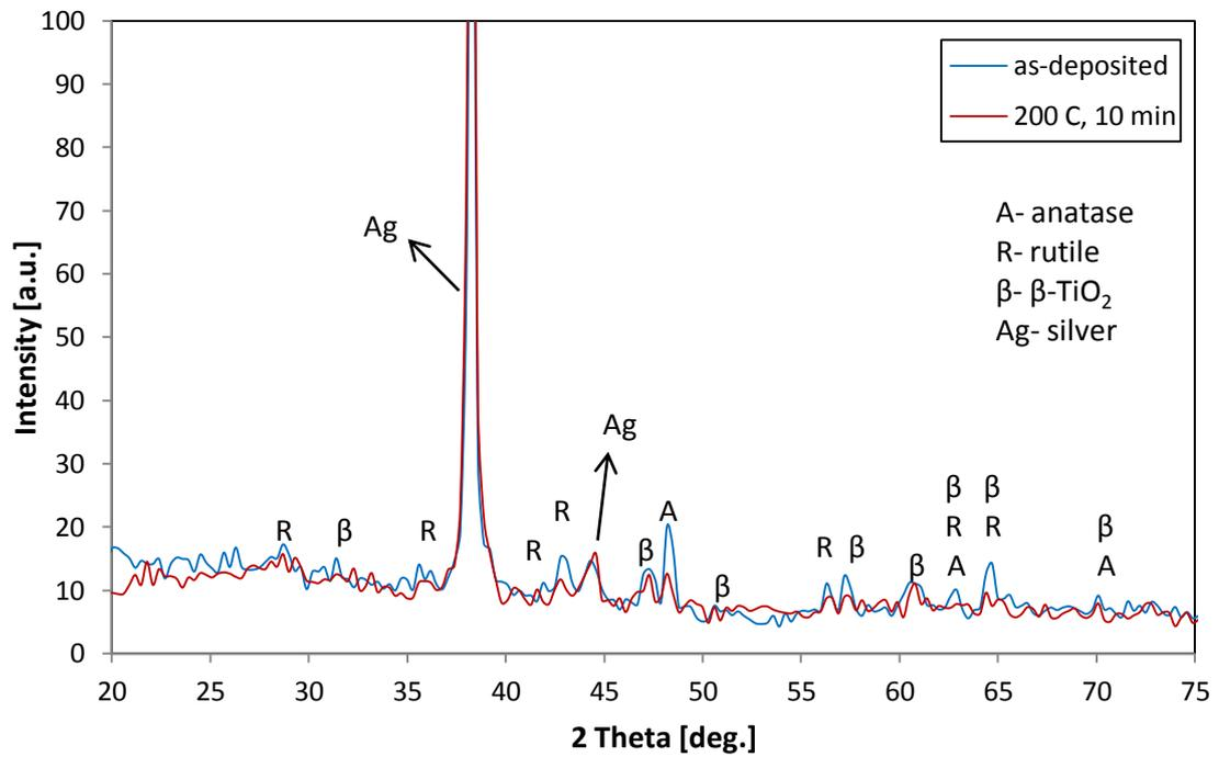
Figure 10.20: XRD diffractograms collected from TiO<sub>2</sub> as-deposited sample and annealed at 200°C for 10 minutes.
