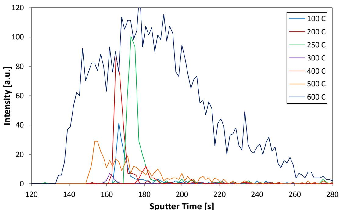
Figure 14.14: Silver distribution in  $\text{Si}_3\text{N}_4/\text{Ag}/\text{Si}_3\text{N}_4$  coatings deposited on glass and annealed at the range of temperatures of 100-600°C for 5 minutes.
