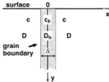
Figure 6.8: Schematic geometry from the Fisher model of grain boundary diffusion, where  $\delta$  is the GB width,  $D_b$  is the GB diffusion coefficient,  $D$  is the volume diffusion coefficient and  $C$  and  $C_b$  represents concentration of the diffusion atoms in the volume and in the boundary respectively. [102]
