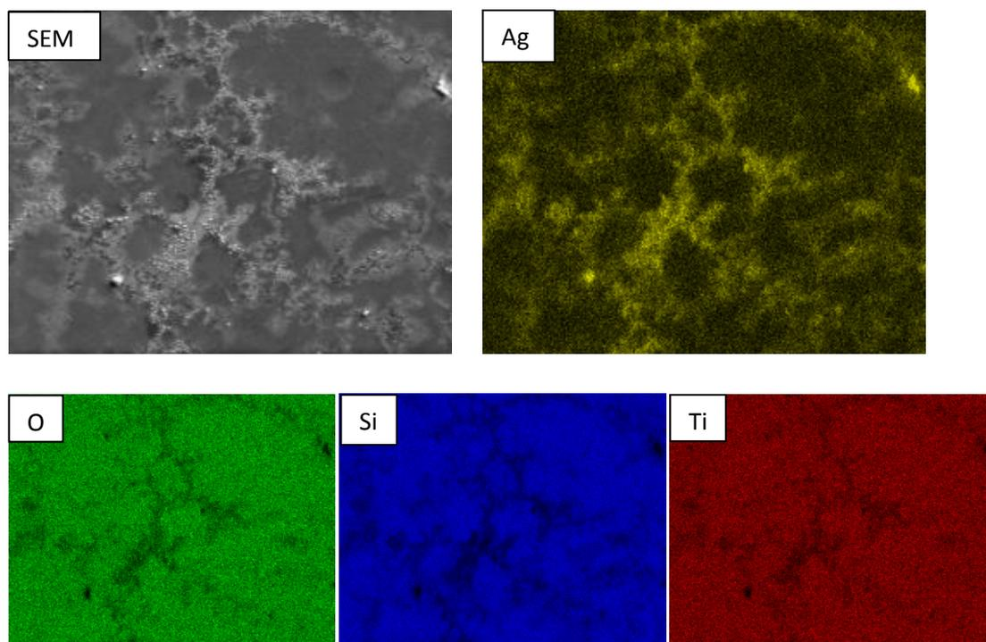
Figure 14.10: EDX mapping performed onto  $\text{TiO}_2/\text{Ag}/\text{TiO}_2$  sample deposited onto Si wafer substrate. Comparing EDX results with the surface image (SEM), it can be seen that the white clusters agglomerated onto the surface are silver atoms.
