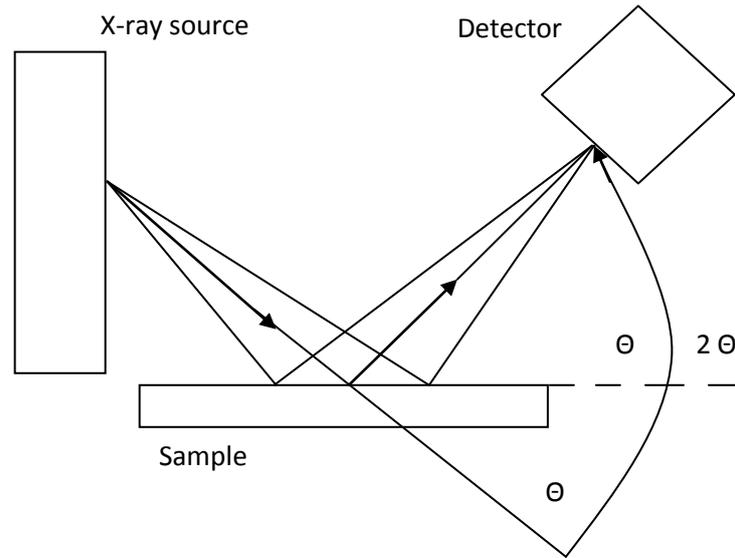
Figure 8.3: Schematic representation of simplified XDR apparatus.
