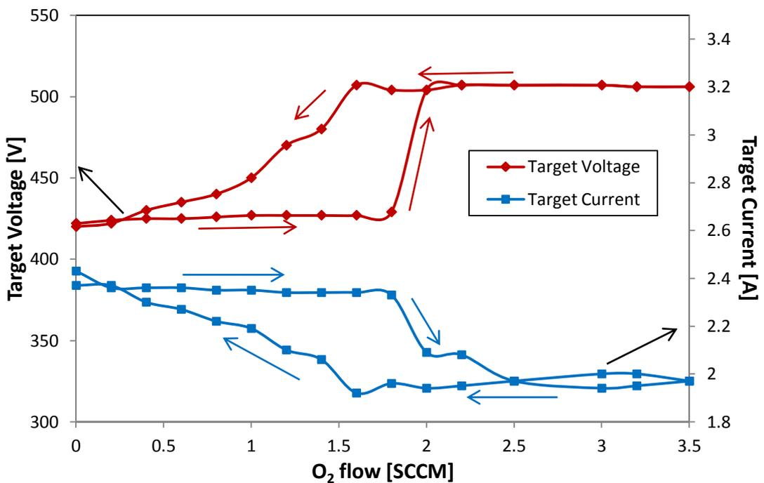
Figure A.2: The effect of the oxygen flow rate on cathode voltage and current in TiO<sub>2</sub> operated under 50 rpm magnetron speed. The arrows show the way in which the data was acquire.
