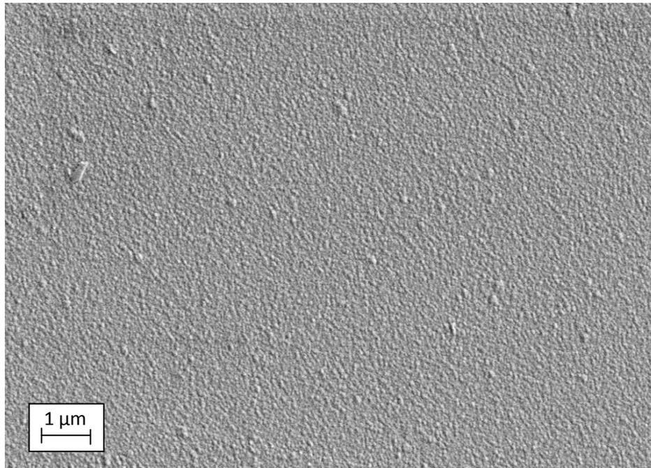
Figure 13.12: SEM micrograph of the top surface of silicon nitride sample 7 deposited onto float glass, post-deposition annealed at 650°C for 5 minutes.
