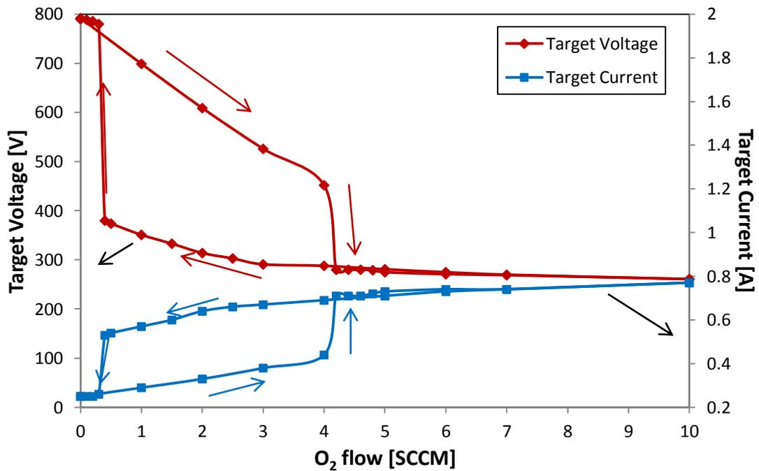
Figure B.1: The effect of the oxygen flow on the cathode voltage and current in AZO sputtered from FFE magnetron at stationary mode. The arrows show the way in which the data was acquired.
