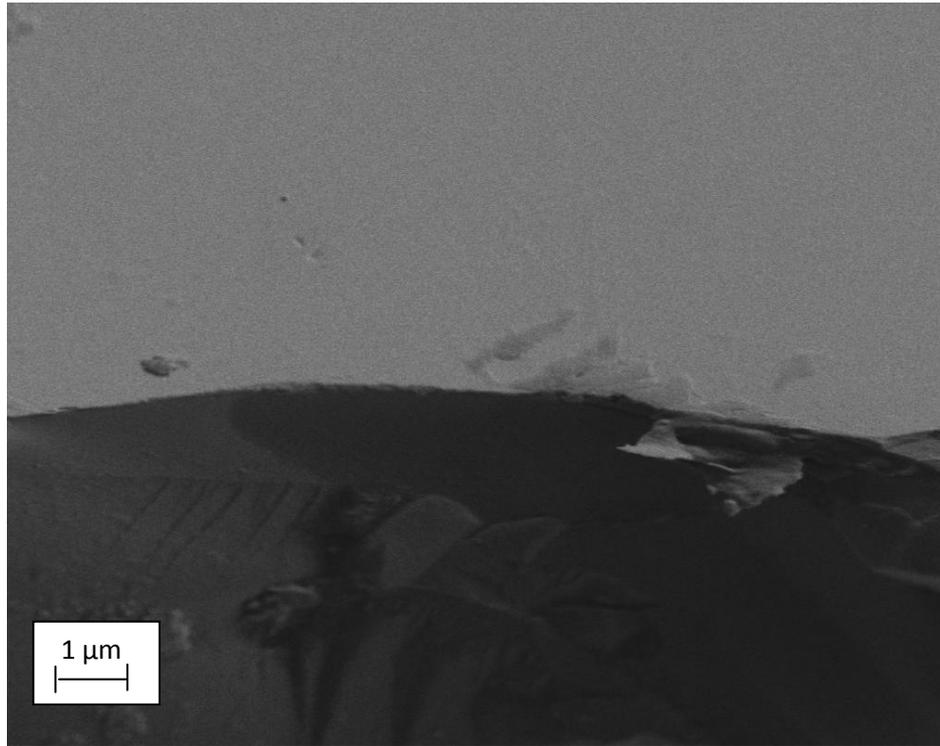
Figure 12.3: SEM micrograph of the fracture section of zinc stannate samples 10 deposited onto float glass.
