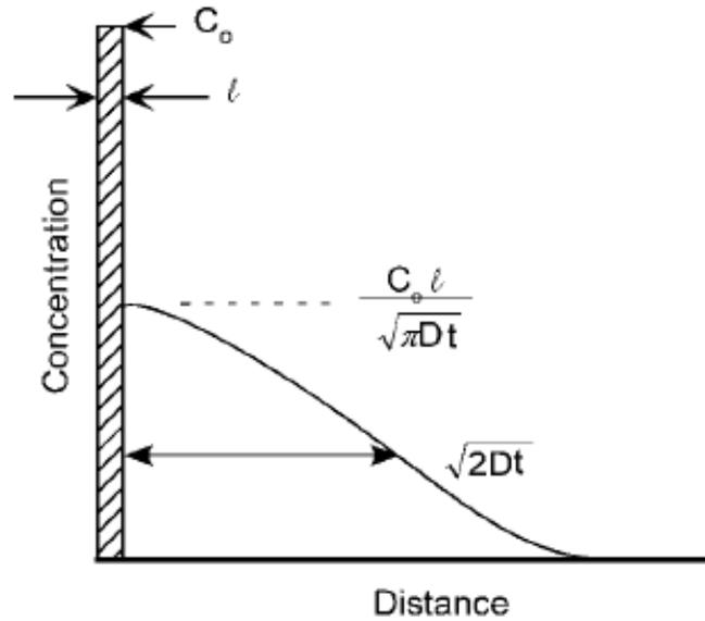
Figure 6.2: Gaussian profile of the thin layer deposited onto substrate surface after sufficient time. [95]
