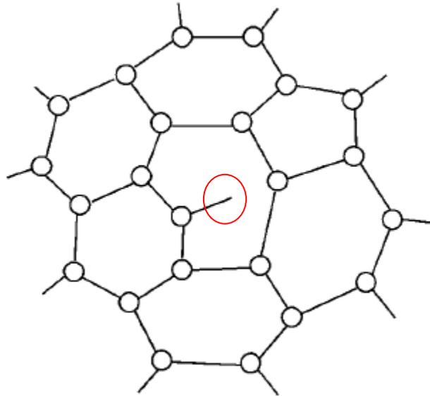
Figure 6.7: Dangling bond in an amorphous structure network. [95]
