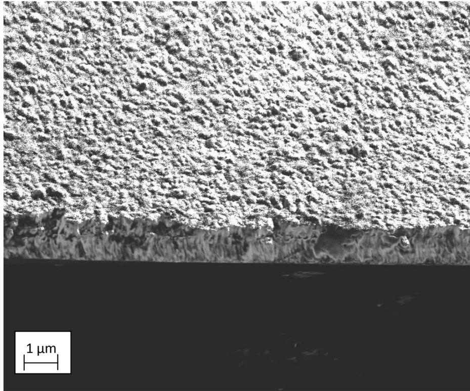
Figure 11.5: SEM image of the fracture section of AZO sample 5 deposited onto float glass substrate.
