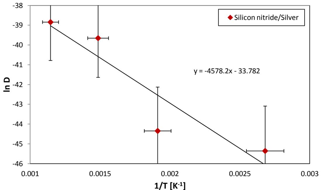
Figure 13.19: Arrhenius dependency between diffusion and annealing temperature obtained from selected silicon nitride/silver sample annealed at the temperature range of  $100\text{-}600^\circ\text{C}$ .
