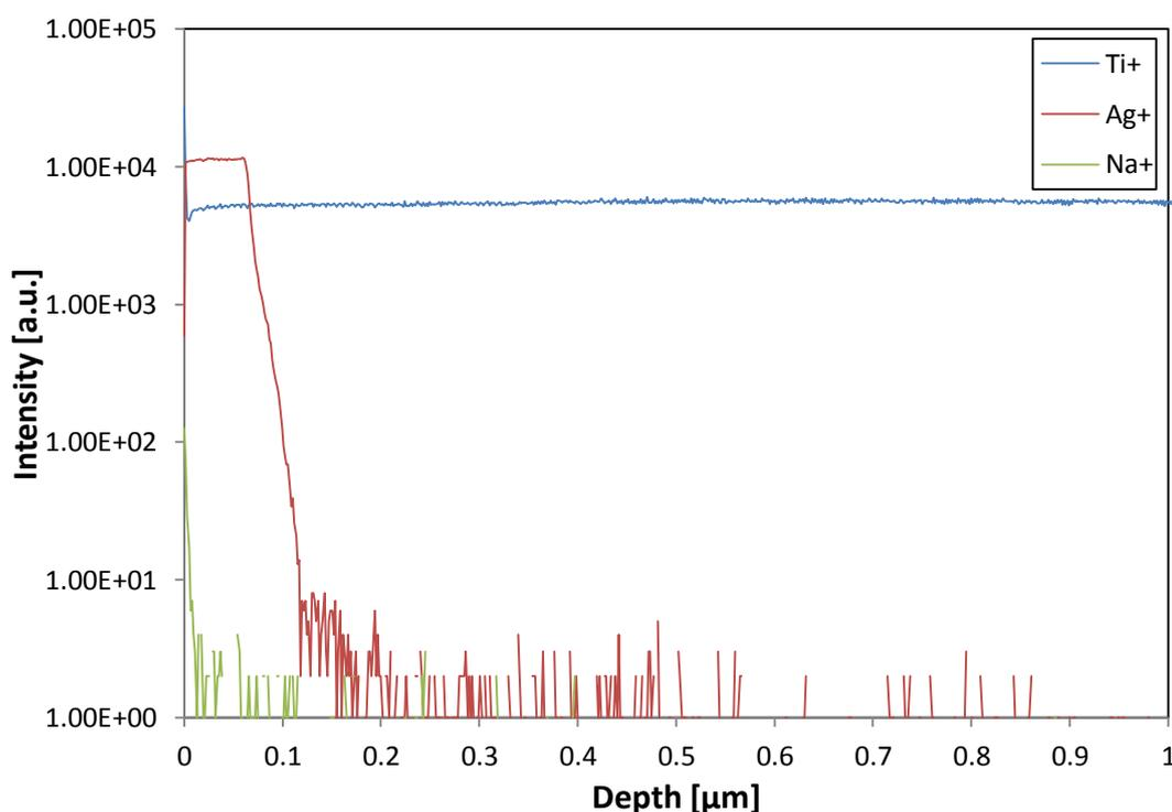
Figure 10.24: SIMS depth profiling of as-deposited Ag/TiO<sub>2</sub>/glass sample, referred to a standard sample in the text.
