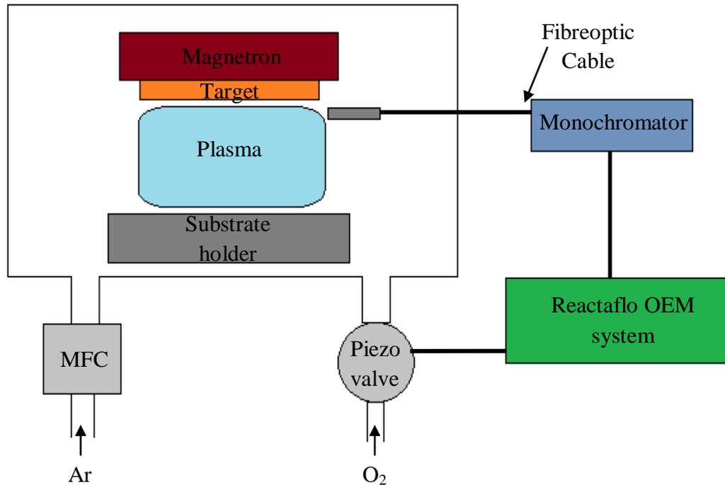
Figure 4.12: Diagram represents OEM layout system.
