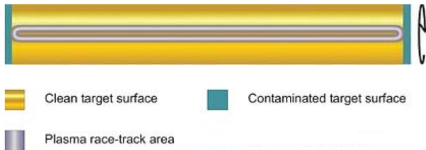
Figure 7.4: Schematic representation of cylindrical rotatable target.
