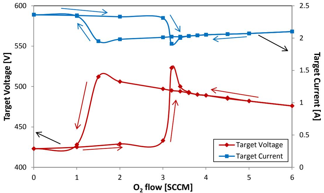
Figure A.1: The effect of the oxygen flow on cathode voltage and current in TiO<sub>2</sub> operated under stationary mode using FFE magnetron design. The arrows show the way in which the data was acquire.
