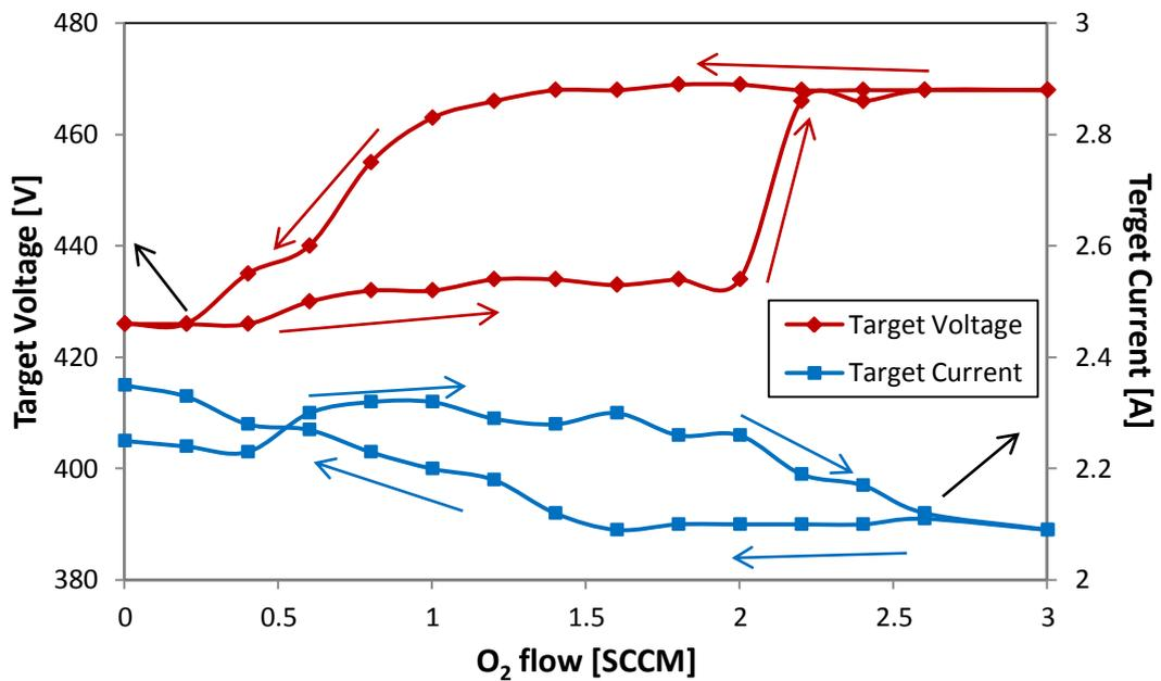
Figure A.4: The effect of oxygen flow rate on cathode voltage and current in TiO<sub>2</sub> sputtered from FFE magnetron rotating at 300 rpm speed. The arrows show the way in which the data was acquire.
