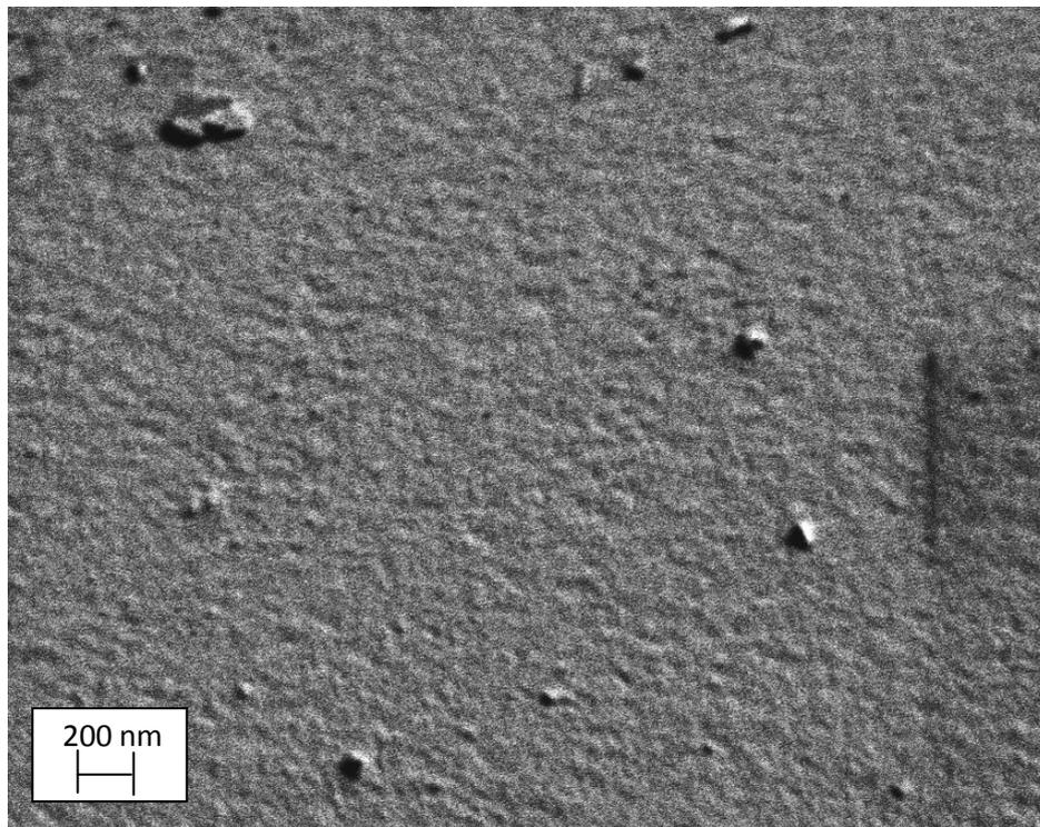
Figure 11.2: SEM image of the top surface of Al-doped ZnO sample 2, deposited onto float glass substrate.
