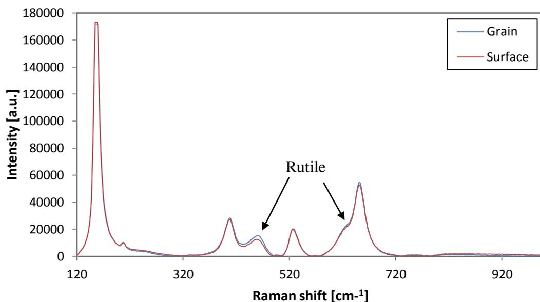
Figure 10.17: Raman images of sample annealed at 800°C, red- obtained from surface, blue- from grain.
