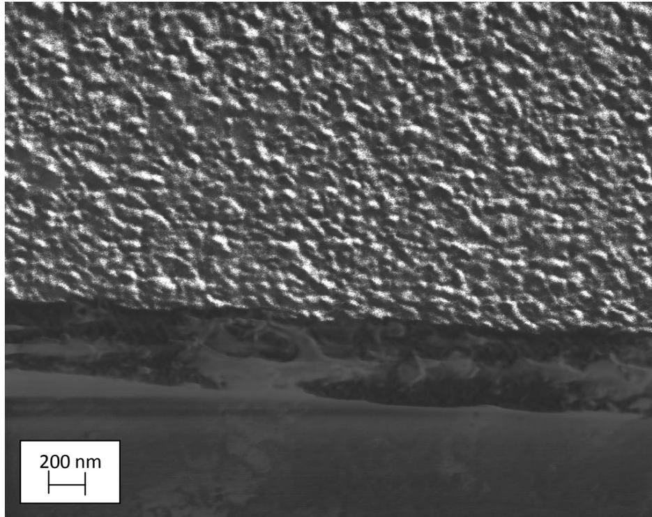
Figure 11.1: SEM micrographs of the fracture section of AZO sample 1 deposited onto float glass substrate.
