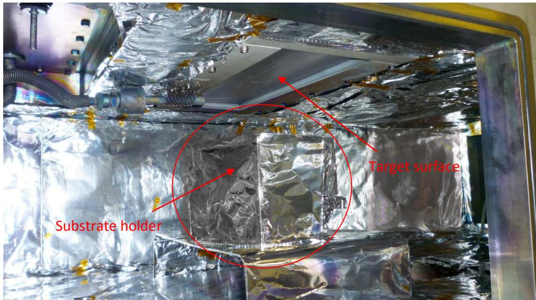
Figure 9.1: Picture shows the substrate holder placed directly under the magnetron in the Large Area coating chamber.
