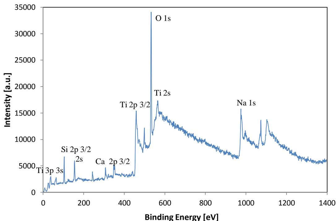
Figure 10.32: XPS spectrum collected for sample 6.1 after reaching the TiO<sub>2</sub>/glass layer interface.
