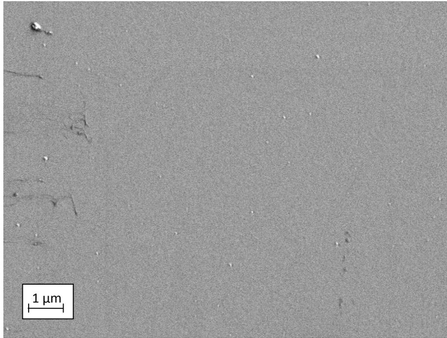
Figure 13.7: SEM micrograph of the top surface of the as-deposited silicon nitride sample 1, deposited onto float glass substrate.
