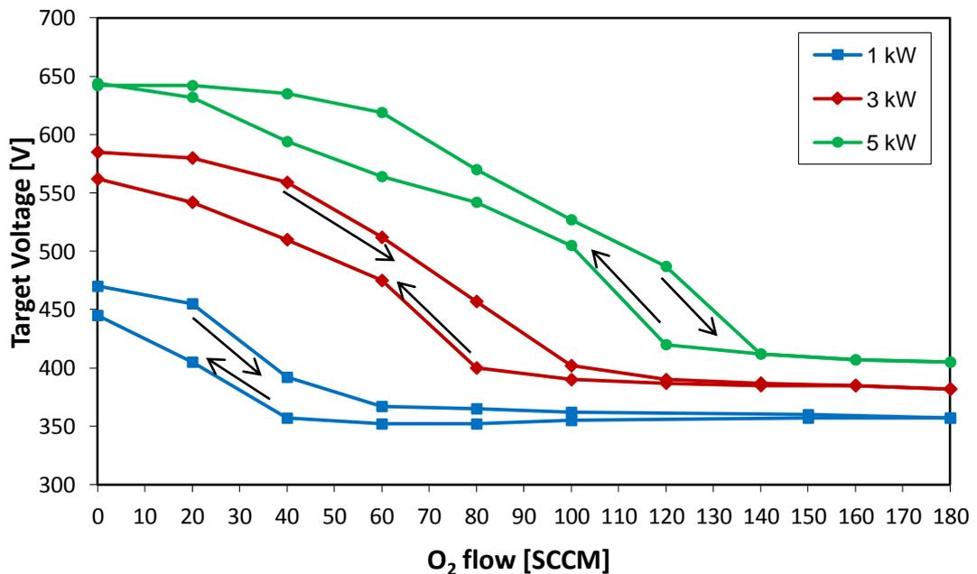
Figure C.3: The effect of the oxygen flow on target voltage in zinc stannate sputtered from dual cylindrical rotatable magnetrons in AC mode and constant powers of 1, 3 and 5 kW. The arrows show the way in which the data was acquired.
