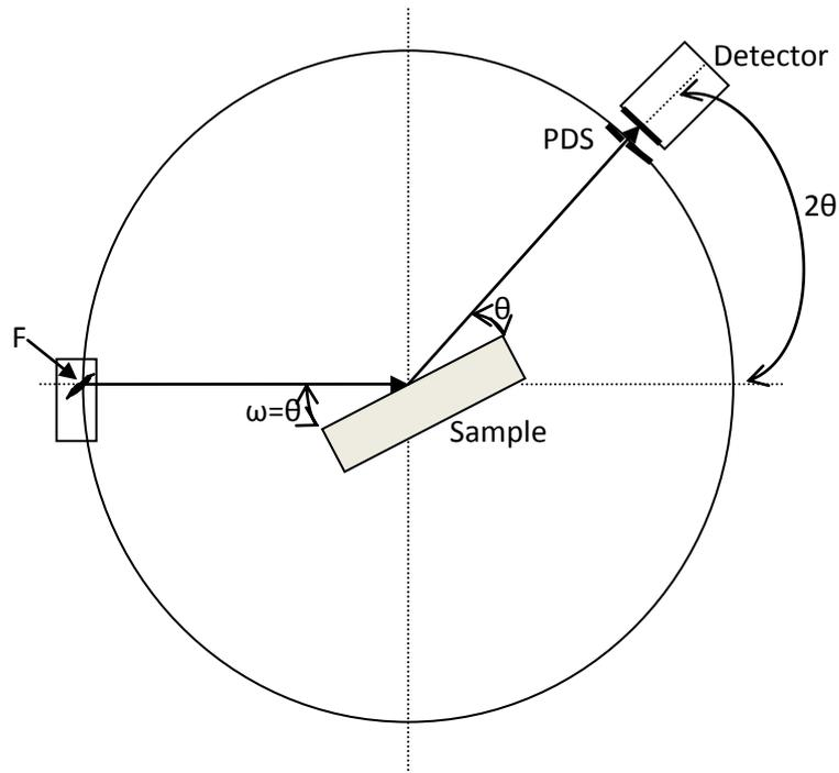
Figure 8.4: Schematic representation of XRR instrument, where the incident angle  $\omega$  equals outgoing angle  $\theta$  and the reflected intensity of  $2\theta$  angle is measured. The anode focus, F of the tubes lies on the detector circle, which is fixed through the detector slit, PRS (programmable receiving slit).
