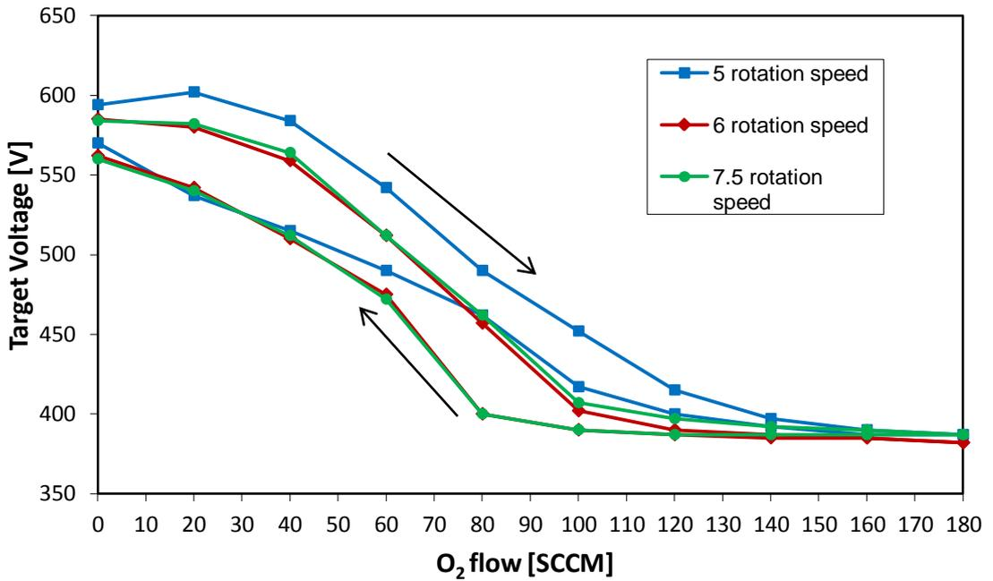
Figure C.4: The effect of the oxygen flow on the target voltage in rotatable magnetron design driven in AC mode at constant power of 3 kW and different rotation speed of 5, 6 and 7.5. The arrows show the way in which the data was acquired.
