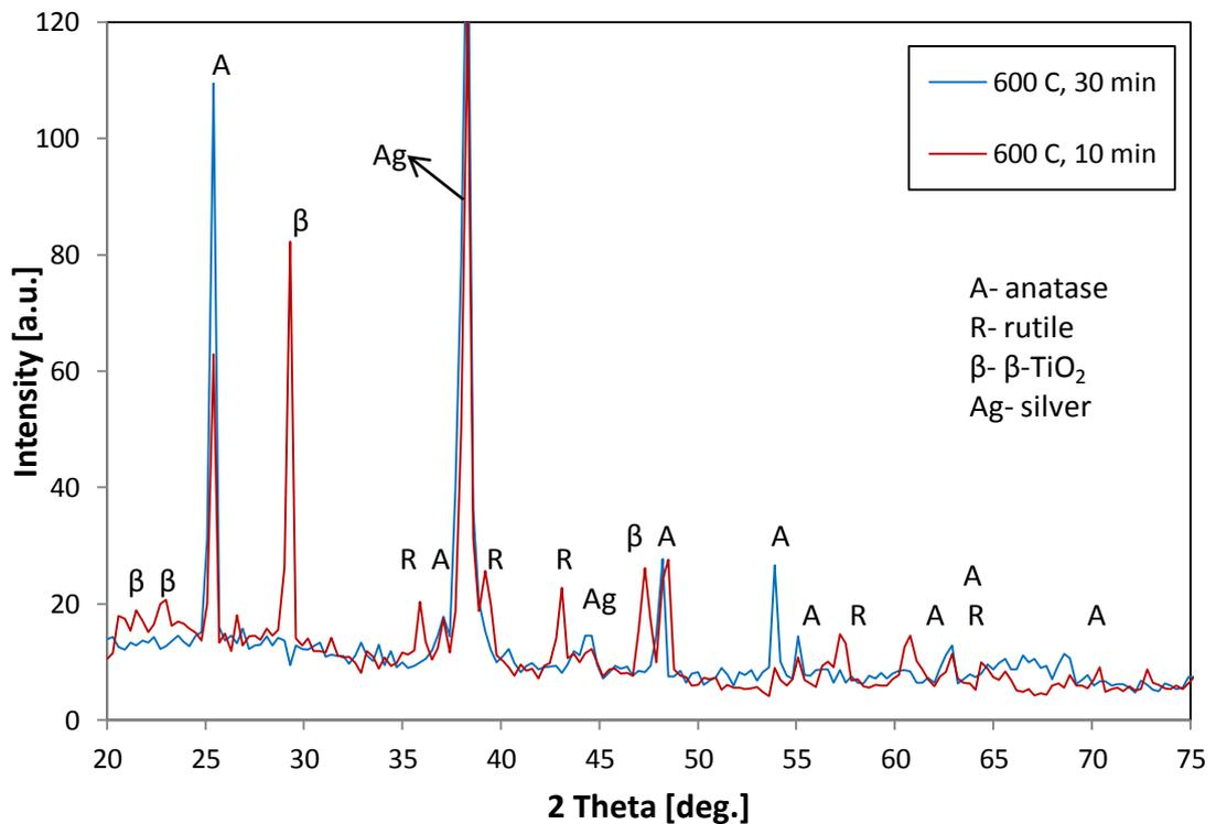
Figure 10.22: XRD diffractograms collected from samples annealed at 600°C for 10 and 30 minutes respectively.
