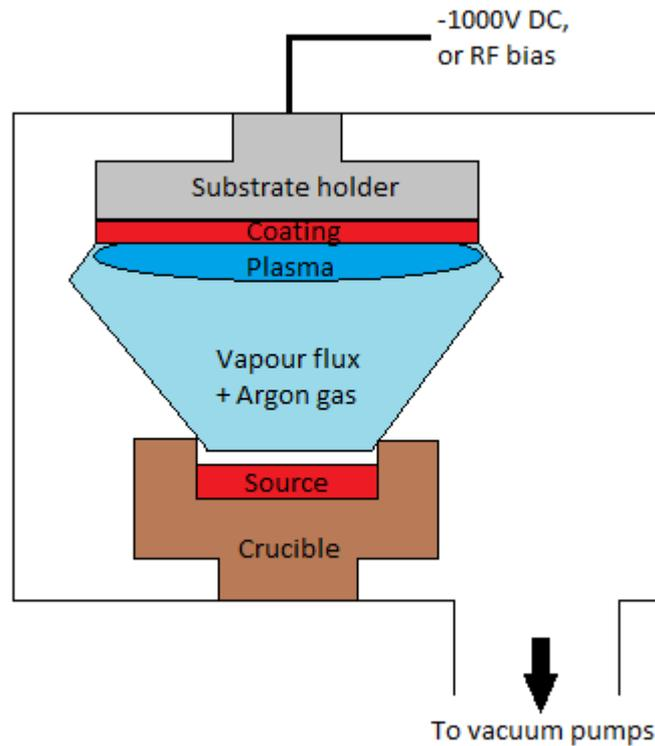
Figure 4.2: Schematic representation of typical ion plating system.
