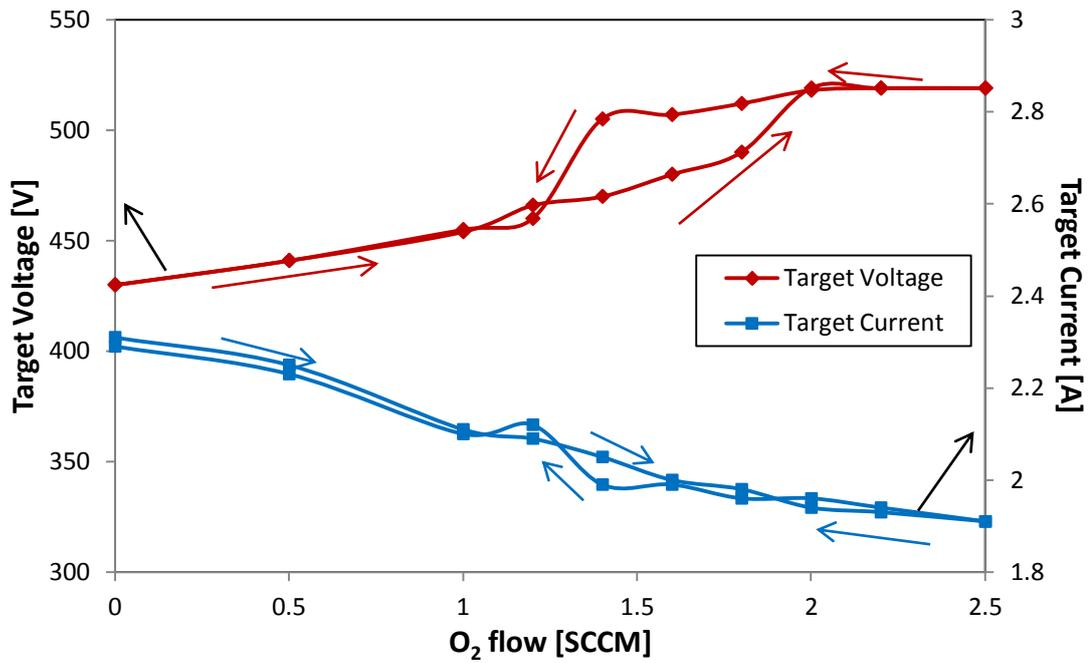
Figure A.3: The effect of the oxygen flow on cathode voltage and current in TiO<sub>2</sub> sputtered under the magnet rotation of 150 rpm. The arrows show the way in which the data was acquire.
