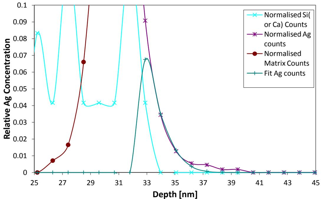
Figure 11.13: An example of an analytical solution to Fick's second law for silver atoms in the Al-doped ZnO sample 1.1.
