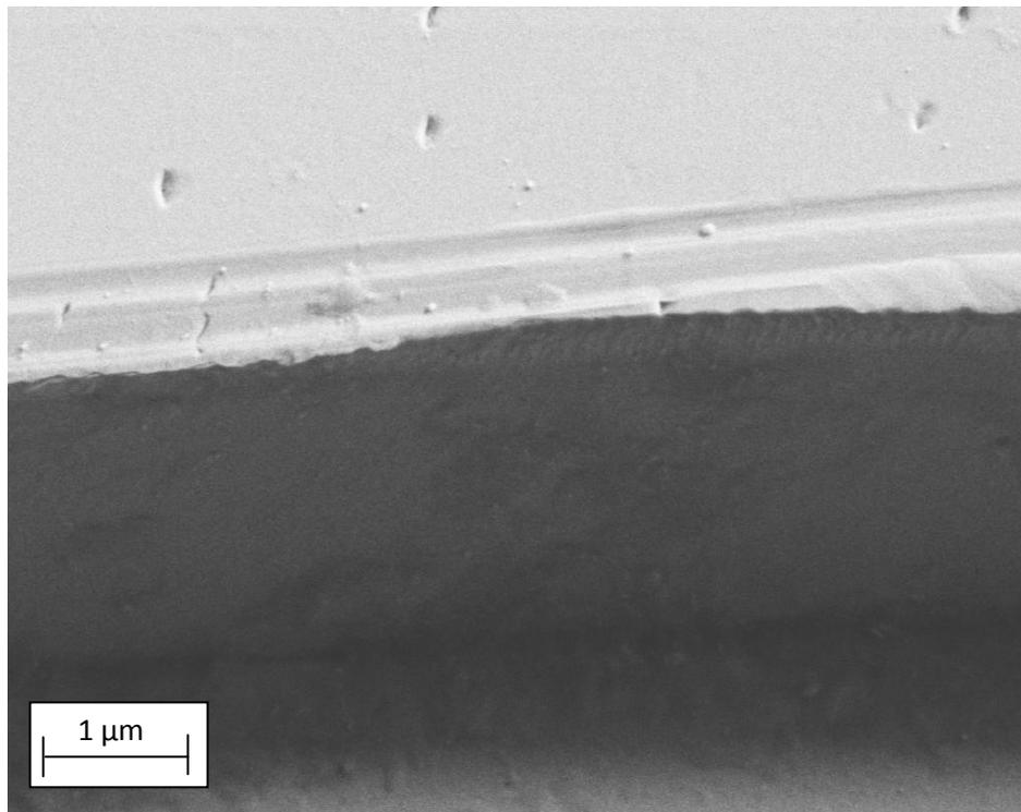
Figure 10.7: SEM image fracture view collected from titania sample 2, deposited onto float glass substrate.
