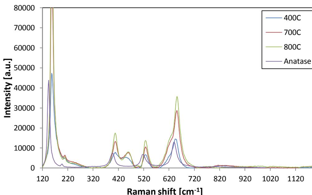
Figure 10.3: Raman spectra of TiO<sub>2</sub> coatings annealed over the range of temperatures from 400 to 800° C aligned with the anatase standard.
