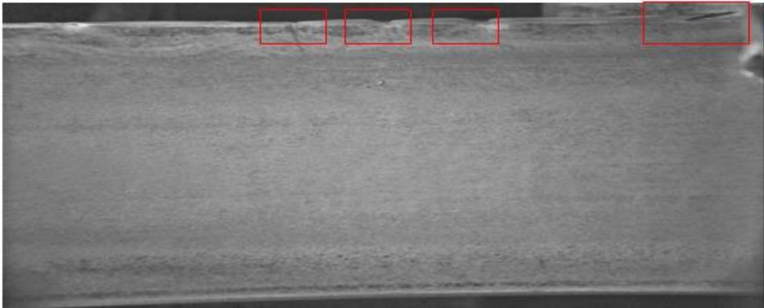
*Figure 5.1: Rail image with rolled in scrap*
