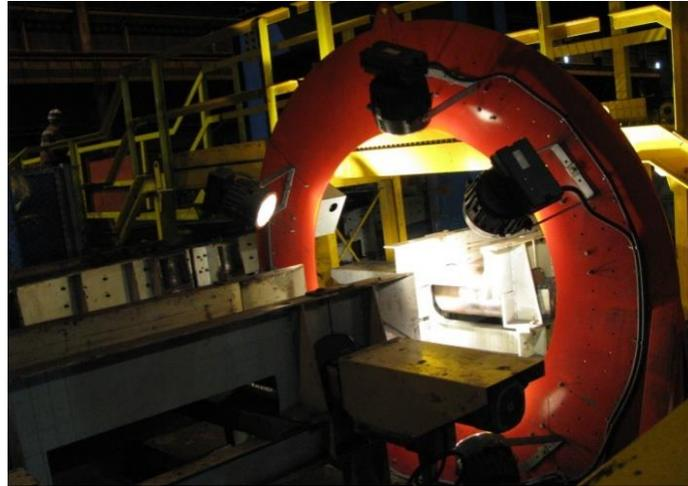
*Figure 3.1: On-site area scans cameras and high intensity lighting.*
