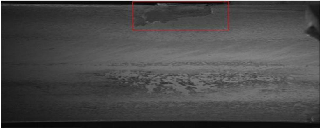
*Figure 5.2: Rail image with rolled in scrap defect highlighted by a red rectangle.*
