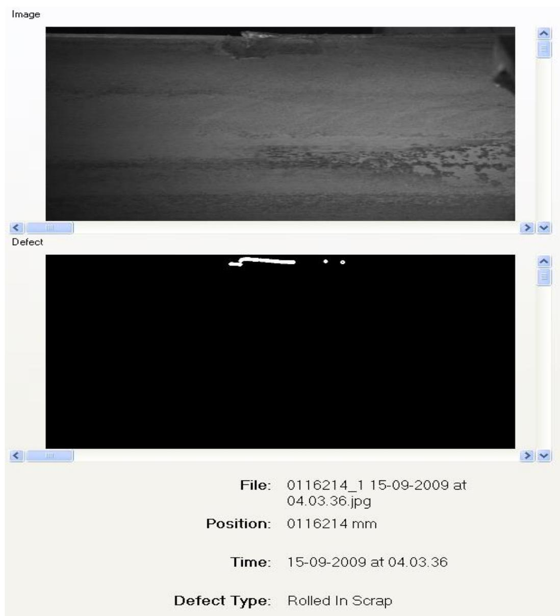
*Figure 7.3: Screen shot from the software interface for Rolled in scrap detection.*
