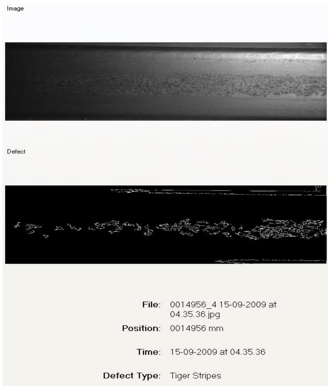
*Figure 7.5: Screen shot from the software interface for Tiger Stripe type defect detected.*
