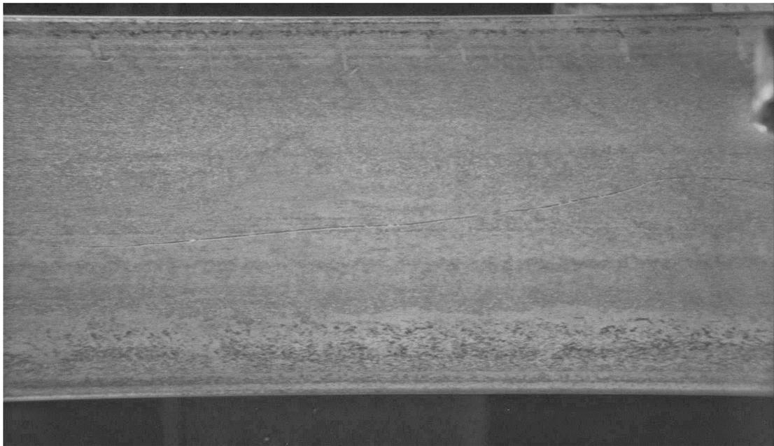
*Figure 3.10: Original rail image with wire defect captured by camera 1.*
