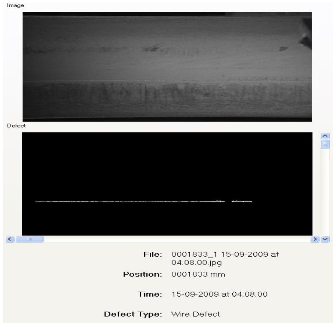
*Figure 7.6: Screen shot from the software interface for Wire defect detected.*
