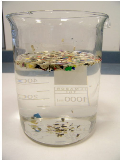
Figure 29: Image of a second float-sink separation process. The denser, non-polyolefinic fraction can be seen at the bottom of the beaker.
