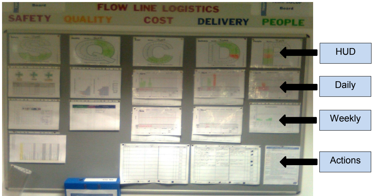
Figure 6.7: Example SQCDP Team Board Airbus Broughton Plant (2001-2006)
