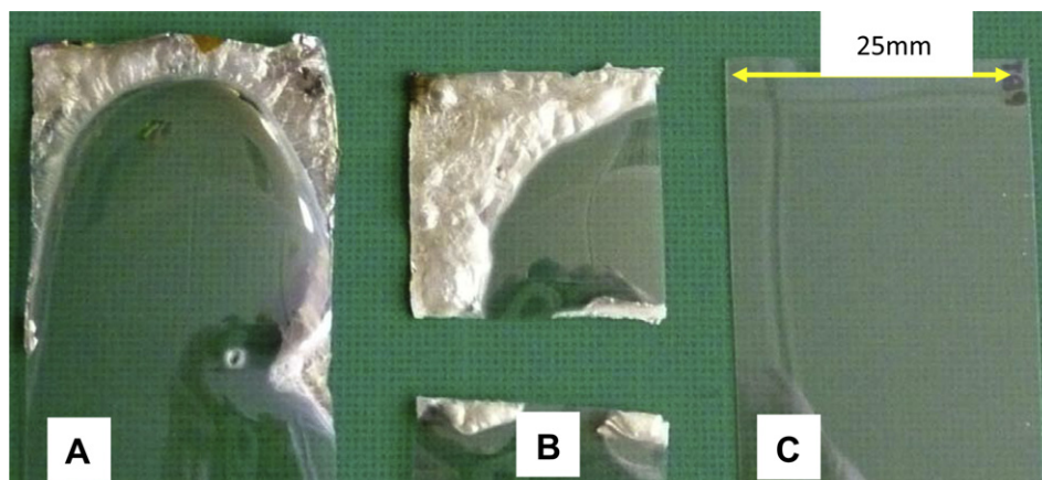
Fig. 1. PET samples coated with titania via reactive magnetron sputtering operating in A) pulsed DC mode; B) HiPIMS mode with a Synex power supply; and C) HiPIMS mode with a Huettinger power supply.
