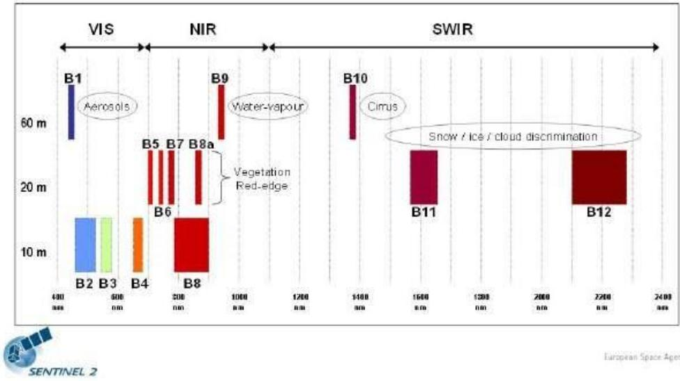
Figure 4b: Sentinel-2 wavebands and resolutions
