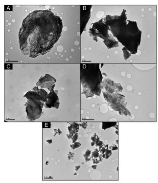
Fig. 2 Structural characterisation of the graphene lateral flakes via TEM; (A) AO-1, (B) AO-2, (C) AO-3, (D) AO-4 and (E) C1. Note that the scale bar is 2  $\mu$ m in all images.
