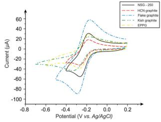
**Fig. 3** Typical cyclic voltammetric profiles recorded using graphite paste electrodes. Redox probe: 1 mM hexaammineruthenium( $\mid \mid$ ) chloride/0.1 M KCl. Scan rate: 100 mV s $^{-1}$ .
