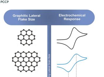
Fig. 4 A schematic depicting the trends observed and reported herein. It is evident that, as the graphitic lateral flake size ( $L_{\rm a}$ ) decreases, an increase in electrochemical reactivity is observed, with increases noted in  $k^{\rm O}$  values obtained and a reduction in the  $\Delta E_{\rm P}$ .
