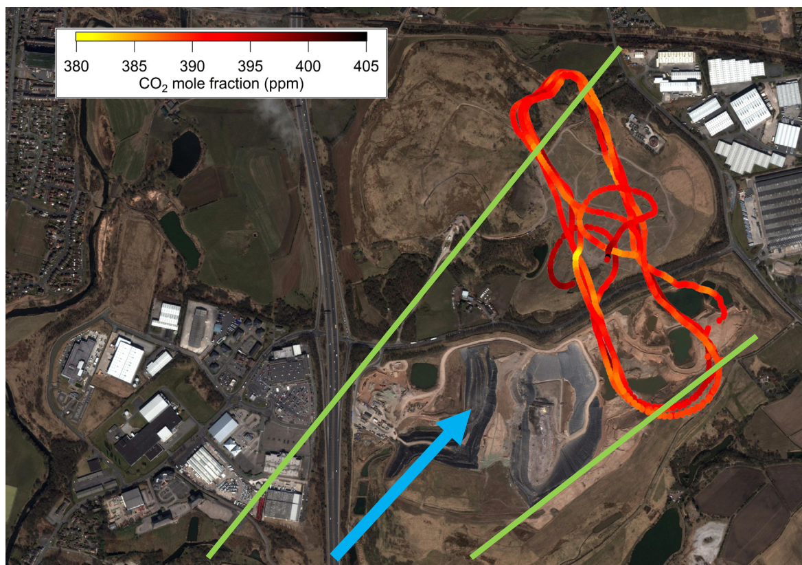
Fig. 3. Flight track and CO 2 concentrations (scaled to color legend) on 5 March 2015 at Site 1. A blue arrow shows mean wind direction on the day and green lines illustrate the expected landfill plume extent. Map data: Google, < http://www.earth.google.com >, DigitalGlobe, 2012 [accessed 12 March 2016]. (For interpretation of the references to colour in this figure legend, the reader is referred to the web version of this article.)
