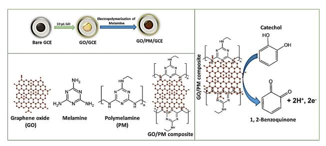
**Scheme 1** Schematic representation for the fabrication of GO/PM modified electrode and its electro-oxidation towards CC.
