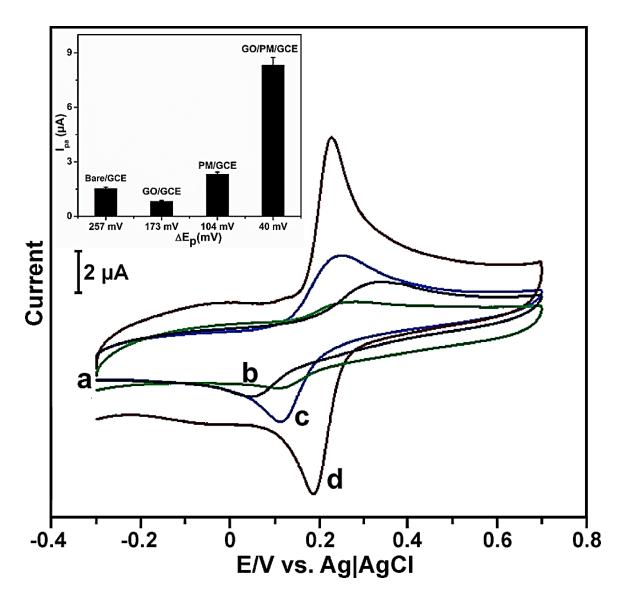
**Figure 2** Cyclic voltammetric response of bare (a), GO (b), PM (c) and GO/PM composite (d) modified GCEs in 100 μM CC containing pH 7 at a scan rate of 50 mV s<sup>-1</sup>. Inset shows the catalytic activity (oxidation peak current response and peak to peak separation) of different modified electrodes towards CC. Error bar relative to five measurements.
