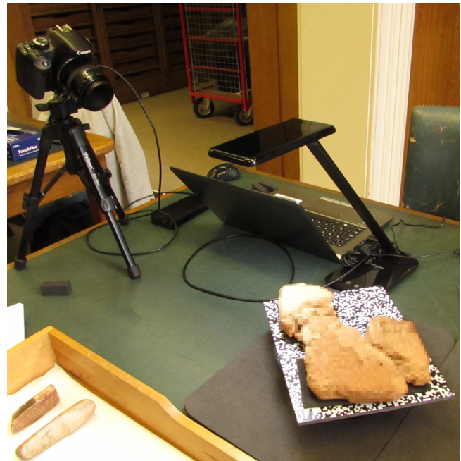
Fig. 4. Tablet C_1 (pixelated) prior to acquisition at the British Museum. The turntable is almost completely hidden underneath the 200 mm \times 280 mm calibration plate made especially for this tablet.
