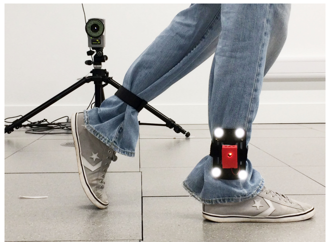
Figure 3: Rigid plates with retroreflective markers and IMU units worn in the motion capture lab.
