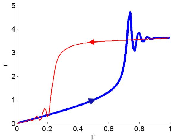
Fig. 6. Plot of  $\Gamma$  versus  $r$  for the nonlinear pendulum. Note the ringing at the ends of the hysteresis loop. The steady states in this case are stable limit cycles. The parameters used in this case were  $k = 0.1$ ,  $\beta = 1$ ,  $\alpha = 0.1$ , and  $\omega = 1.25$ , where  $\Gamma$  is linearly ramped up from  $\Gamma = 0$  to  $\Gamma = 1$ , and then ramped back down again.
