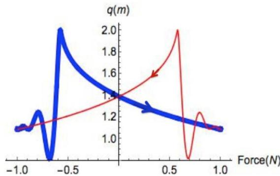
Fig. 4. Input-output map between the vertical force,  $F$ , and the horizontal displacement,  $q$ , given by equation (5) at a low frequency  $\omega = 0.05$ (r/s). Note the ringing at the ends of the hysteresis loop. The parameters used are  $k = 1$  (N/m),  $m = 1$  (kg),  $c = 1$  (Ns/m),  $m_{\text{bar}} = 0.5$  (kg),  $l = 1$  (m) and  $F = \sin(\omega t)$ .
