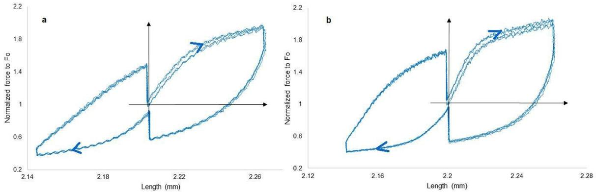
Fig. 16. Four cycles of normalized force vs length, for two different fibres a and b with  $f = 0.25 \text{ (s}^{-1}\text{)}$ .
