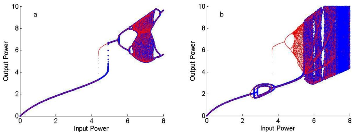
Fig. 8. Bifurcation diagram of the SFR resonator, the power  $|A|^2$  was ramped up from  $0 \text{ W m}^{-2}$  to  $8 \text{ W m}^{-2}$ , and back down again. (a) When  $B = 0.15$ , the isolated counter-clockwise hysteresis loop (bistable region) is followed by a region of period-doubling to chaos. (b) When  $B = 0.24$ , instabilities encroach upon the hysteresis cycle at both ends.
