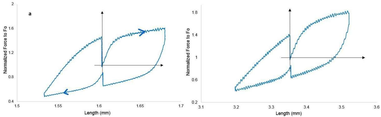
Fig. 14. Normalized force vs length for two different fibres. The input frequency was double that used to produce Figure 13,  $f = 0.25 \text{ (s}^{-1}\text{)}$ .
