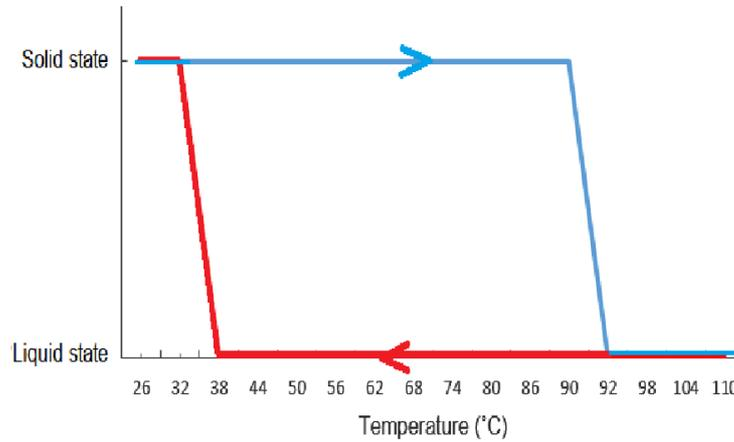
Fig. 1. Clockwise hysteresis cycle between the melting and setting temperatures,  $32^{\circ}$  and  $90^{\circ}$ , respectively, of the agar gel. Whether the agar is solid or liquid at a certain temperature between the melting and gelling states will depend on the previous state of the substance.
