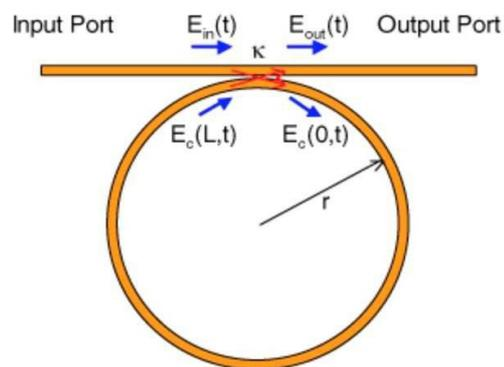
Fig. 7. A schematic of the SFR resonator. The electric fields entering and leaving the fibre ring are indicated. The parameter  $\kappa$  represents the power-splitting ratio at the coupler and  $L$  is the length of the fibre loop.
