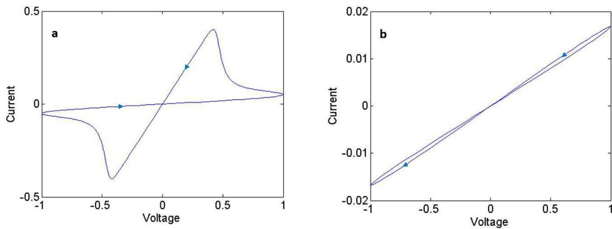
Fig. 9. Pinched hysteresis of a memristor in the  $I - V$  plane. a For low frequencies there is a definite pinched hysteresis. b As the frequency gets higher, the pinched hysteresis degenerates and the memristor acts like a linear resistor. For more details see [Lynch, 2014].
