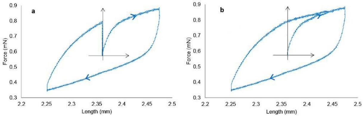
Fig. 11. a Force-length relationship corresponding to Figure 10a. The curve is a hysteresis loop for only one period of the input and for this fiber the origin is where  $F_0=0.58$  (mN) and  $l_0=2.36$  (mm). b A convex clockwise hysteresis loop develops when there is no relaxation at the end of lengthening and shortening.
