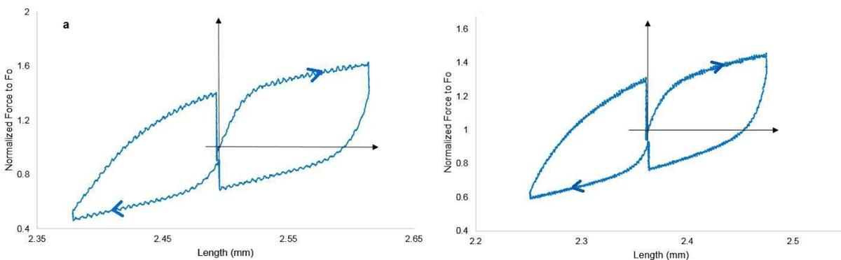
Fig. 13. Normalized force vs length for two different fibres a and b. The input frequency for both examples was  $f=0.125$  ( $s^{-1}$ ). The force produced by the fibres reached different percentages of  $F_0$ .
