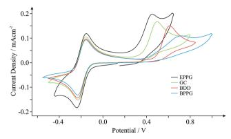
Fig. 1 Cyclic voltammograms obtained in pH 7 PBS (with 0.1 M KCl) containing 0.5 mM NADH and 0.5 mM Ru(NH $_3$ ) $_6^{2+/3+}$  (internal standard) at EPPG (black), GC (green), BDD (red) and BPPG (blue) electrodes. Scan rate shown: 100 mV s $^{-1}$  (vs. SCE).
