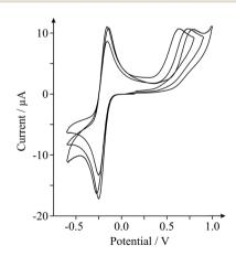
Fig. 3 Cyclic voltammograms obtained in pH 7 PBS (with 0.1 M KCl) containing 0.5 mM NADH and 0.5 mM Ru(NH $_3$ ) $_6^{2+/3+}$  (internal standard) at three different double-layered defect-abundant graphene electrodes to investigate the inter-repeatability. Scan rate shown: 100 mV s $^{-1}$  (vs. SCE).
